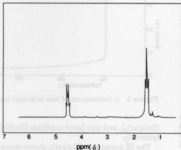
**Figure 7** An H-NMR spectrum of zinc ethyl xanthate.
