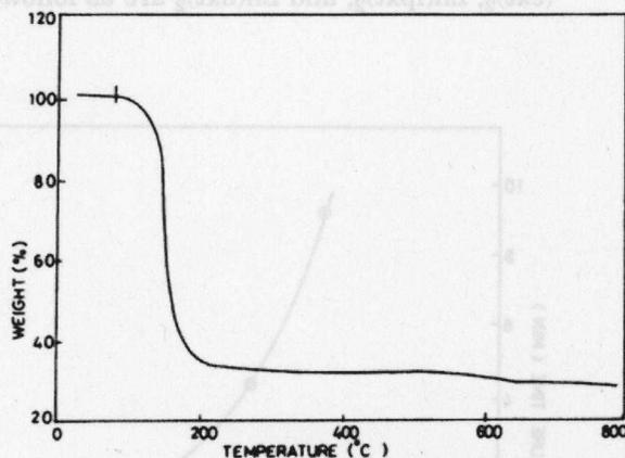
Figure 4 A thermogram of zinc ethyl xanthate.
