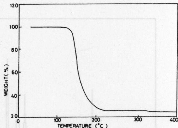
Figure 6 A thermogram of zinc butyl xanthate.
