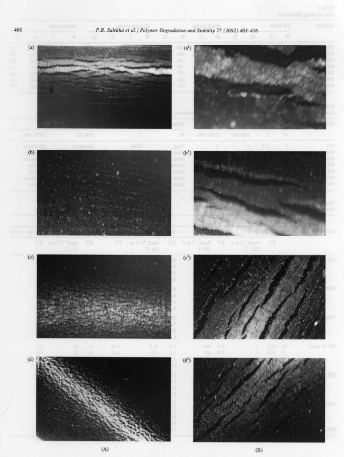
Fig. 1. (A) Ozone crack initiation of NR vulcanizates (a) without antioxidant, (b) with vulkanox 4020, (c) with PIB–PD, (d) with CPW–PD; (B) ozone crack growth after 19 h ( $a^1$ ) without antioxidant, ( $b^1$ ) with vulkanox 4020, ( $c^1$ ) with PIB–PD, ( $d^1$ ) with CPW–PD.
