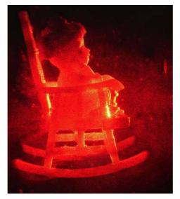
Fig.5.28 The photograph of the hologram recorded and reconstructed using He-Ne laser
