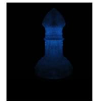
Fig. 6.19 Photograph of the hologram recorded on DCPVA/AAm
