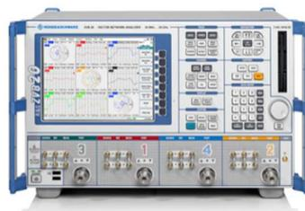
**Fig 3.5** Rhode & Schwartz ZVB 20 used in measurement
