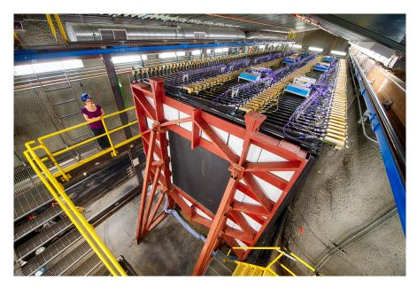
Figure 3.9: The NOvA ND view from where the beam enters the detector. A person is seen on the right for the scale.
