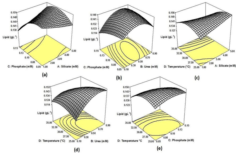
Fig. 4.6 RSM plots of lipid as a function of (a) phosphate and silicate (b) phosphate and urea (c) temperature and silicate (d) temperature and urea (e) temperature and phosphate in MSW medium
