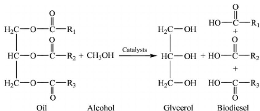
**Fig. 1.2** Transesterification reaction of microalgal lipids resulting in biodiesel and byproduct of glycerin (Ahmed et al., 2015)
