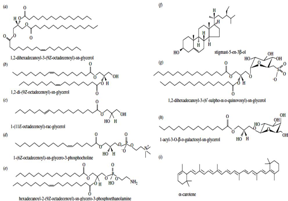
**Fig. 1.3** Chemical structures of most common representatives from seven lipid classes: (a) triacylglycerides; (b) diacylglycerides; (c) monoglycerides; (d) phospholipids; (e) sterols; (f) sulpholipids; (g) glycolipids; (i) carotenoids (courtesy www. LipidMAPS.org)
