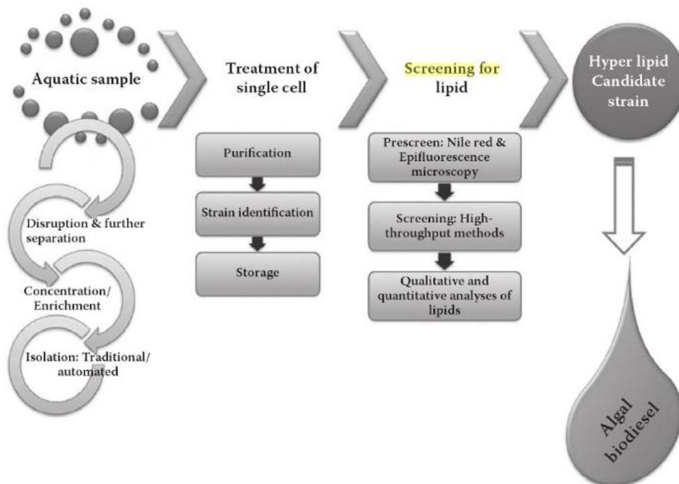
**Fig. 3.1** Schematic outline for procedures in bio prospecting of microalgae for biodiesel production (Karthikeyan, 2013)
