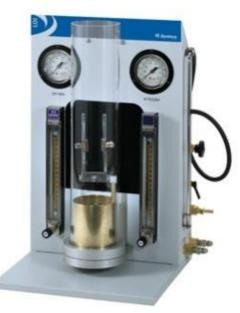
Figure 2.7: Set up for LOI measurement
