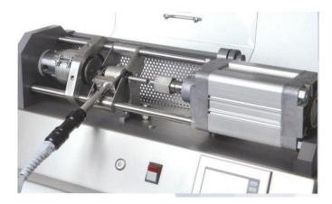
Figure 2.1: DSM Micro 12 cc Injection moulding machine
