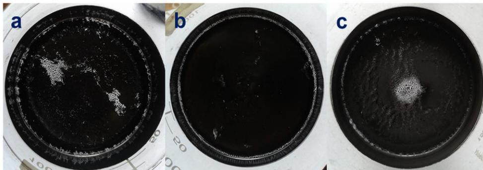
**Fig. 3.A.9** Photographs of MWCNT film formed after drying the aqueous suspensions having MWCNT and VL in different ratios (a) 1: 0.5 (b) 1:1 (c) 1:2
