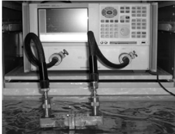
**Fig. 2.3 Set-up for EMI shielding measurement**
