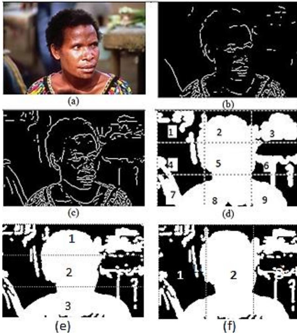
**Figure 3.2** Salient sub-block identification. (a) Original image (b) Edge map after Sobel edge filtering (c) Edge map after edge thresholding / boosting (d) Regions of 3x3 grid (e) Horizontal regions (f) Vertical regions
