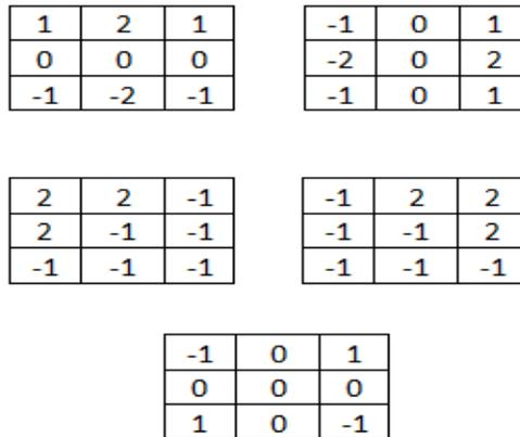
**Figure 4.2** Filters for identifying the five types of edges
