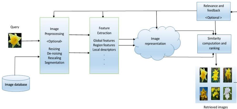
**Figure 2.1** The architecture of a general CBIR system
