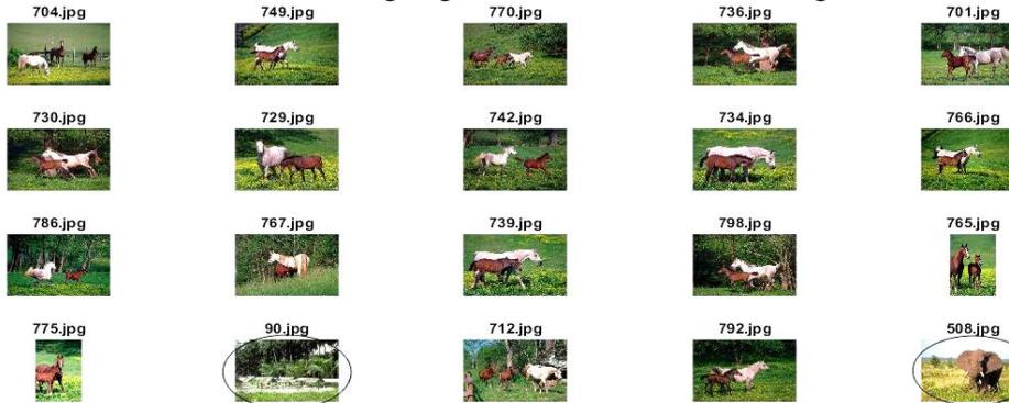
(c) Retrieval using cumulative feature (edge-colour and SURF) based histogram
