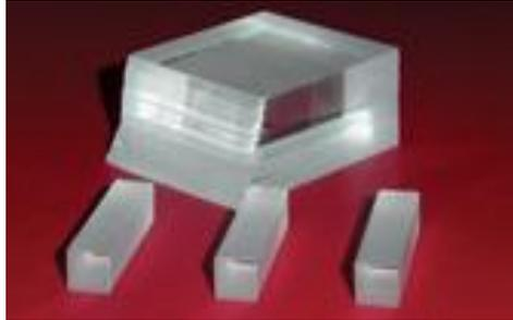
**Figure 1.1: A typical crystal for stimulated Raman scattering**
