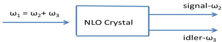
Figure.1.6. Optical parametric oscillator
