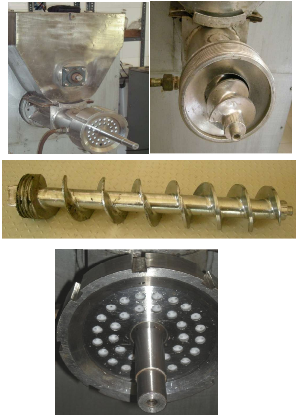
Plate-5. Single screw extruder used for the study
