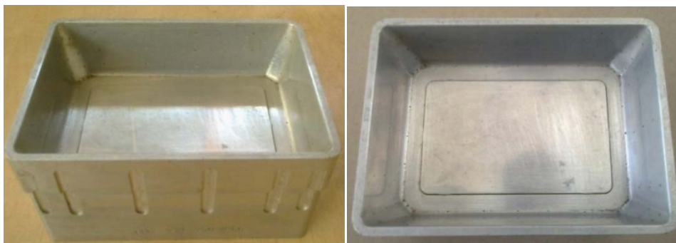
Plate-13. Die used for thermoforming
