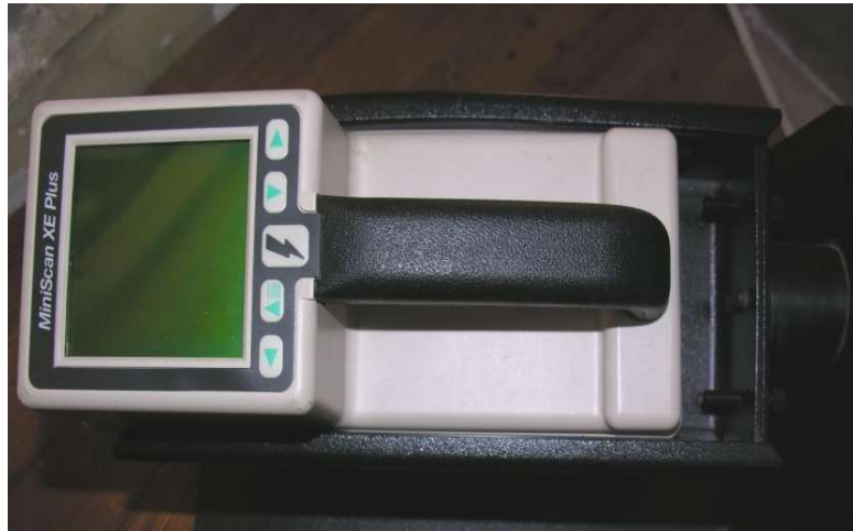
Plate-10. Hunterlab colour measurement device
