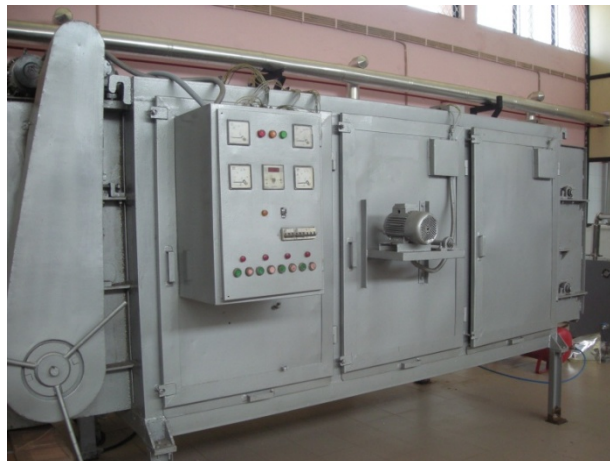
Plate-7. Electrical dryer for drying the extruded noodles
