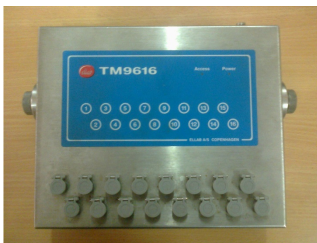
Plate-21. Eval precision thermometer and process value integrator
