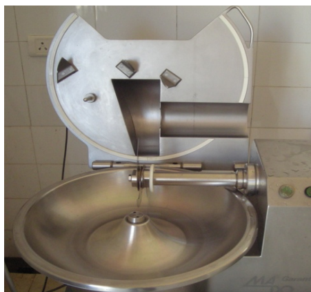
Plate-8. Bowl chopper for mixing the ingredients
