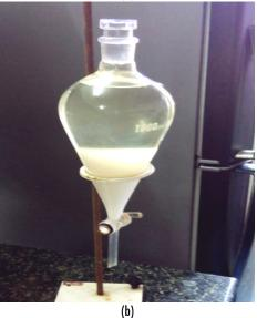
Fig.5.1 a-b: a) Microscale experimental setup for aqueous two phase extraction of *Bacillus* MCCB 242 phytase; b) Macroscale experimental setup for aqueous two phase extraction of *Bacillus* MCCB 242 phytase in 1L separating funnel.
