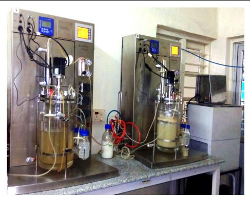
Fig. 5.2: Production of *Bacillus* MCCB 242 phytase in 5L bench top laboratory scale fermentor
