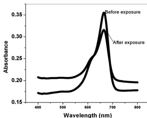
**Figure 3** Optical absorption spectrum of the film C 0.14.
