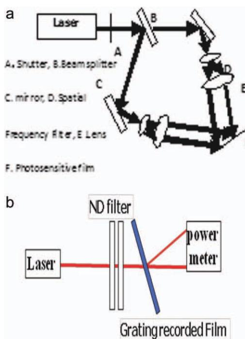
**Figure 1** (a) Double beam setup for recording grating. (b) Experimental setup for diffraction efficiency measurement. [Color figure can be viewed in the online issue, which is available at [wileyonlinelibrary.com](http://wileyonlinelibrary.com).]
