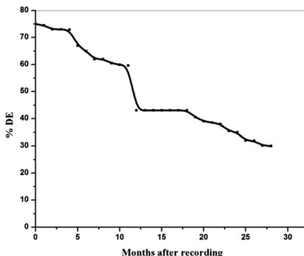
**Figure 7** The DE of grating on C 0.14 film on storage.
