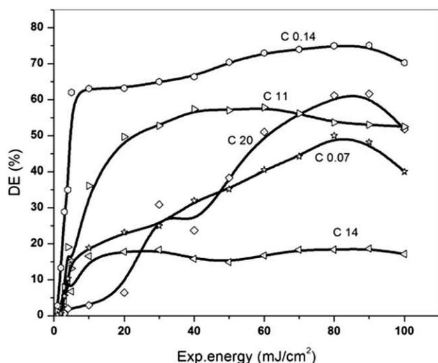
**Figure 2** Exp. energy versus % DE of the films with different dye concentration.
