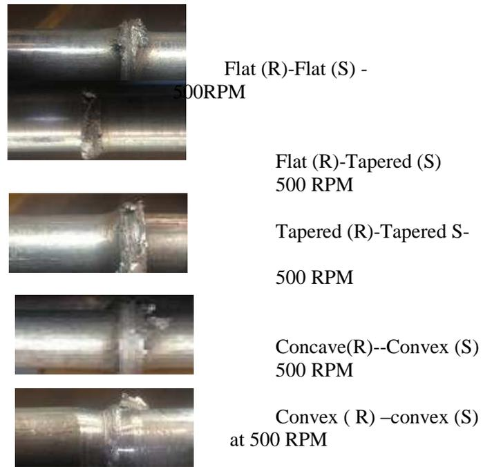
FIGURE . 3 VARIOUS COMBINATIONS OF FRICTION WELDED JOINTS OBTAINED
