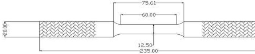
FIGURE 4. STANDARD SPECIMEN FOR TENSION TEST
