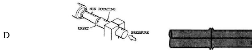
Rotary friction welded joint is formed.
