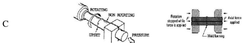
When metal in the joint zone reaches plastic state due to high temperature and heat generation, because of friction, rotation is stopped and axial pressure is increased instantly.
