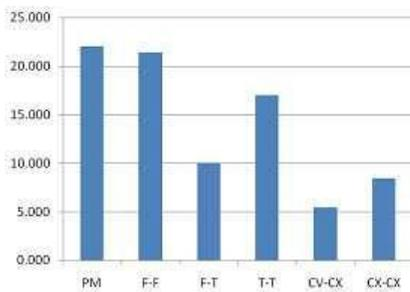
FIGURE 7. PERCENTAGE ELONGATION OF FW JOINTS (AT 500 RPM)
