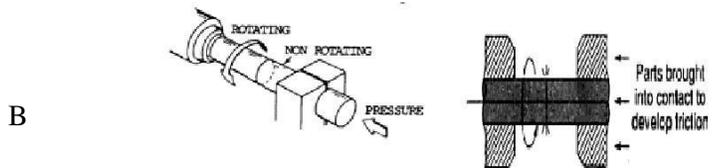
Heat is generated at the contact interface due to friction.
