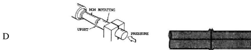
Rotary friction welded joint is formed.
