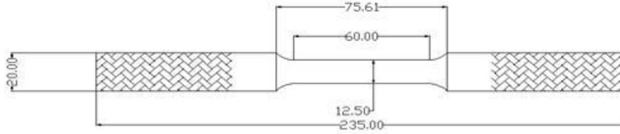
FIGURE 4. STANDARD SPECIMEN FOR TENSION TEST
