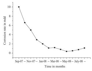
Fig. 2. Corrosion rate of brass samples in the Vembanad estuary for different exposure periods.
