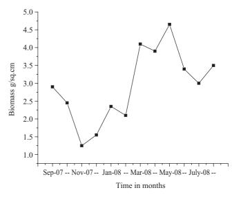
Fig. 3. Biomass settlement on brass samples in the Vembanad estuary for different exposure periods.
