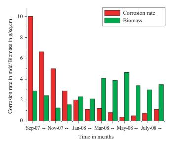
Fig. 4. Comparison of corrosion rate and biomass of brass samples with time in the Vembanad estuary.
