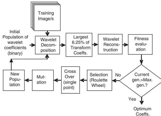
Figure 1. Block diagram of the evolutionary algorithm (GA) for optimising cdf9/7 lifting coefficients for FIC.
