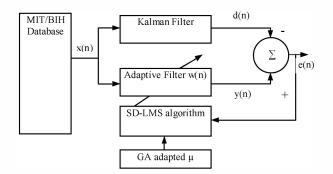
Fig. 1 The proposed SD-LMS configuration for BW removal.
