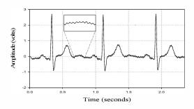
Fig 4. ECG Corrupted with 60Hz PLI
