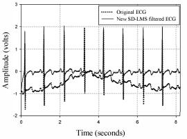
Fig. 2. Results obtained for the removal of BW with the new SD-LMS
