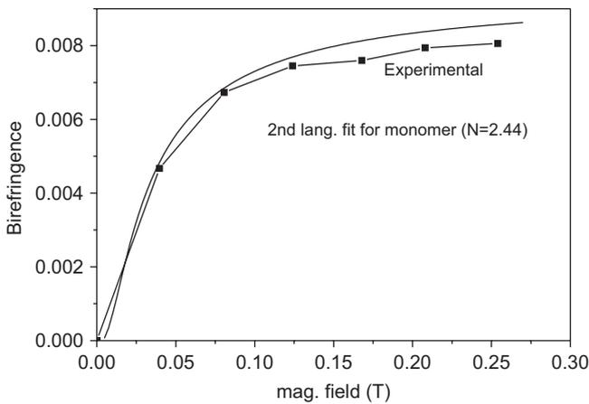
Fig. 9. Representative Langevin curve fitting and experimental birefringence values (fit for  $N = 2.44$ ) for ball-milled  $Ni_xFe_{1-x}Fe_2O_4$  ( $x = 0.1$ ).
