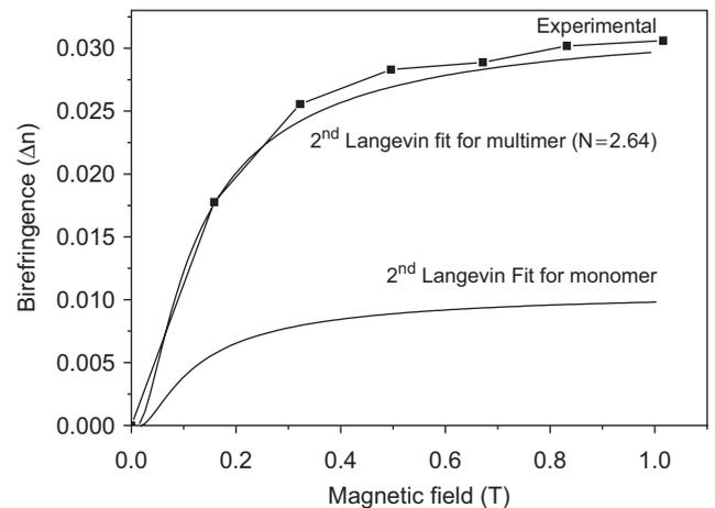
Fig. 10. Langevin curve fitting and experimental birefringence values (fit for multimer  $N = 2.5$ ) for ball-milled  $Ni_xFe_{1-x}Fe_2O_4$  ( $x = 0.1$ ).
