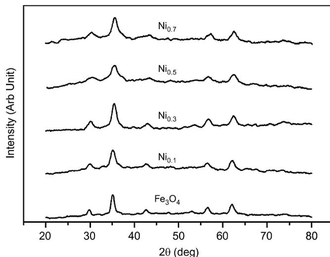
Fig. 2. XRD spectrum of ferrofluid samples  $\text{Ni}_x\text{Fe}_{1-x}\text{Fe}_2\text{O}_4$ .
