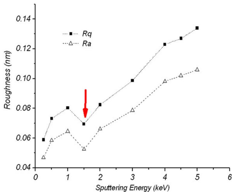
**Figure 2**  $R_a$  and  $R_q$  for FLG as a function of Ar<sup>+</sup> ion irradiation energy. Ranging from 0.25 to 5 keV.
