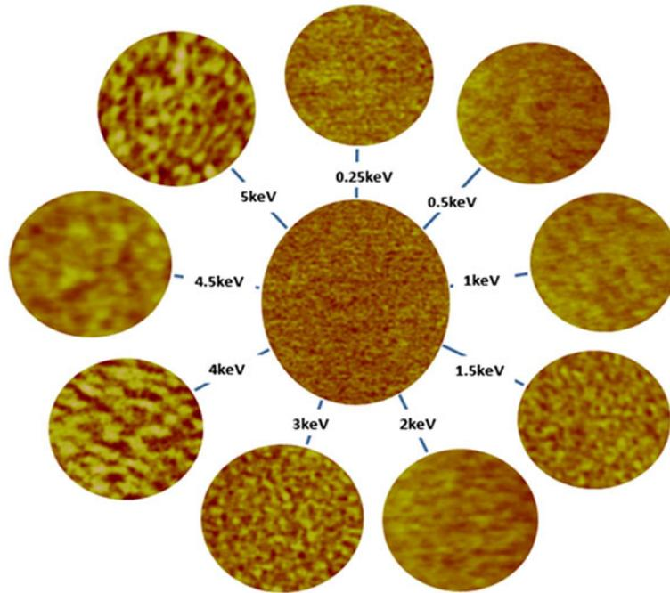
**Figure 1** Sequence of FLG AFM height images as a function Ar<sup>+</sup> irradiation energy 0.25 to 5 keV. The image in the middle was obtained from the un-irradiated FLG sample.
