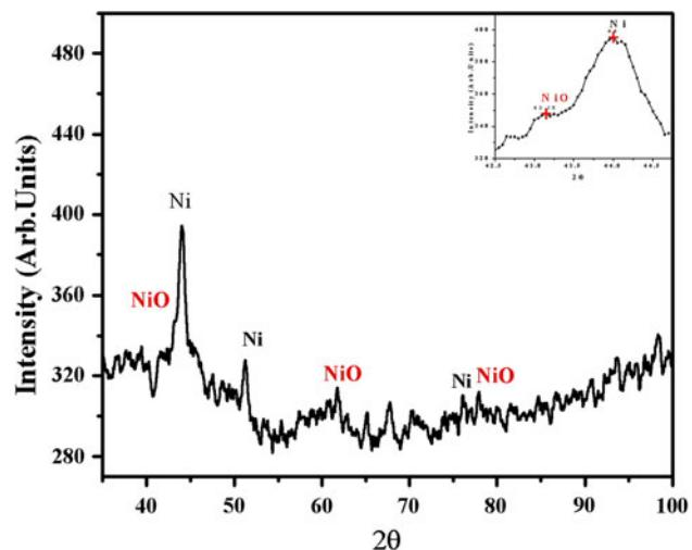
**Fig. 4** XRD pattern of Nickel Polymer composite (WAC-10) (inset enlarged view)
