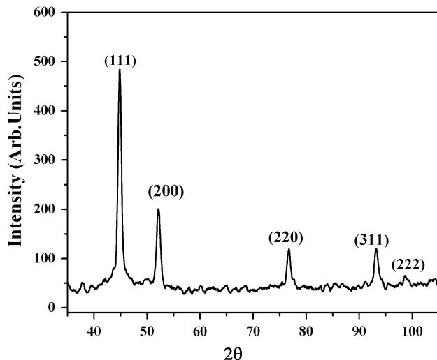
**Fig. 3** XRD pattern of Nickel Polymer composite (SAC-16)
