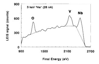
FIG. 1. Typical LEIS spectrum of a V-Nb oxide catalyst (V3Nb, 3 mol% V). The peak areas (above the dashed background lines) are used to quantify the outermost surface composition.
