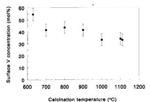
**FIG. 4.** Surface concentration of vanadium in the V10Nb catalyst as determined by LEIS versus the calcination temperature. Calcination at 1100°C was carried out twice for 19 and 24 h, respectively. To distinguish both treatments in the figure, the latter is displayed at 1110°C.
