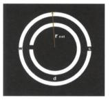
Fig.4. Two Ring SRR with variables External radius ( $R_{ext}$ .), Width of ring(w), Gap between rings(d), Height of substrate (h), Relative permittivity of substrate ( $\epsilon_1$ ), Width of slit in ring(s). Reference dimension chosen is  $R_{ext}$ =6mm; w-0.3mm; d=0.3mm; s=0.3mm; h=1.6mm; and  $\epsilon_1$  =4.4
