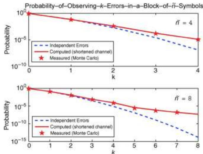
Figure. 7. Error statistics for blocks of 4 and 8 symbols for the channel of Fig. 3(a) with a threshold bias of 36 mV. The results computed analytically based on a shortened channel with  $l=16$  by considering all  $2^{n+l-1}$  symbol patterns match closely the Monte Carlo measurements ( $2.5 \times 10^7$  symbol blocks) for the actual (unshortened) channel. The corresponding result based on the independent-errors assumption is also included.
