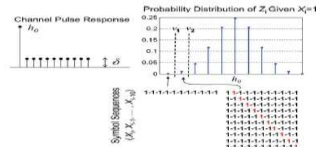
Figure. 2: Simplified pulse response [left] and the corresponding ISI distribution [right]
