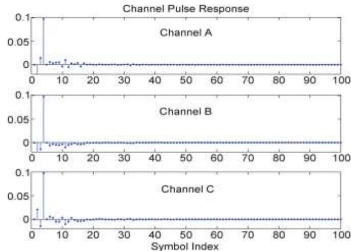
Figure 3. Equalized pulse response of the standard 802.3ap B32 [10] channel operating at 10 Gb/s. Channel A: Actual channel. Channel B: All-positive signature. Channel C: Randomly generated signature.
