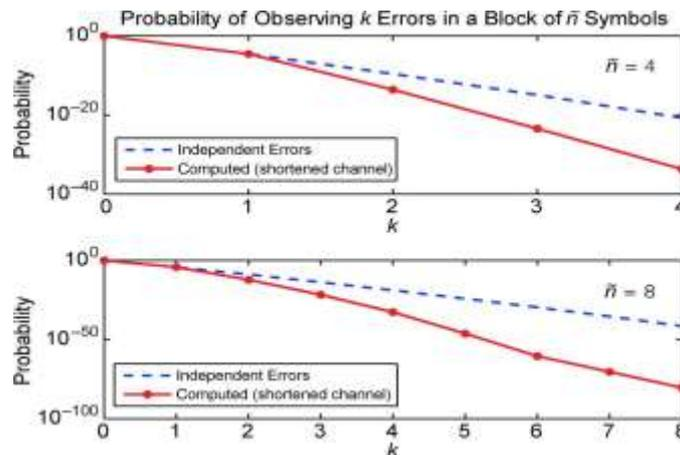
Figure.8. Error statistics for blocks of 4 and 8 symbols for the channel of Fig. 3(a) without the threshold bias of 36 mV. The results computed analytically based on a shortened channel with  $l=16$  by considering all  $2^{n+l-1}$  symbol patterns are compared to the results based on the independent-errors assumption.
