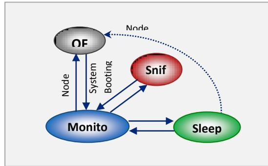
Figure 3 – Sensor Node State Transition
