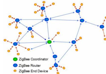
Figure 1-Typical ZigBee WSN – Mesh Architecture
