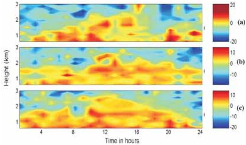
Figure 5 Time-height intensity plot of the hourly averaged Signal to Noise Ratio (SNR) for (a) 23 June, (b) 25 July and (c) 14 August for the year 1999
