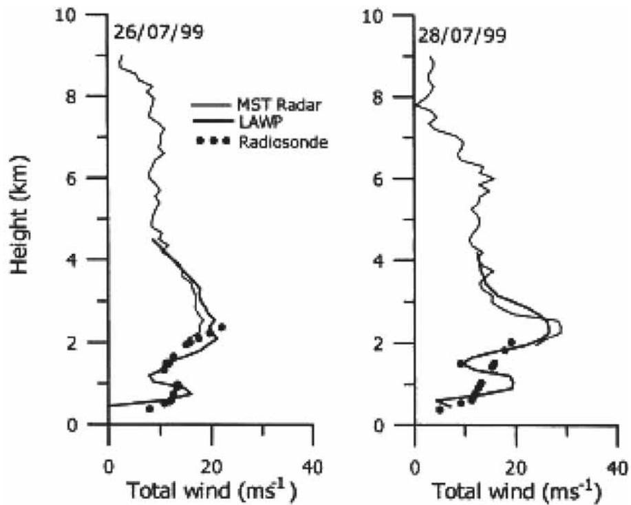
Figure 3 Comparison of wind speed measured by LAW, MST radar and radiosonde on 26 July 1999 (10:30 IST) and 28 July 1999 (16:15 IST). (from Praveena et al 2003)
