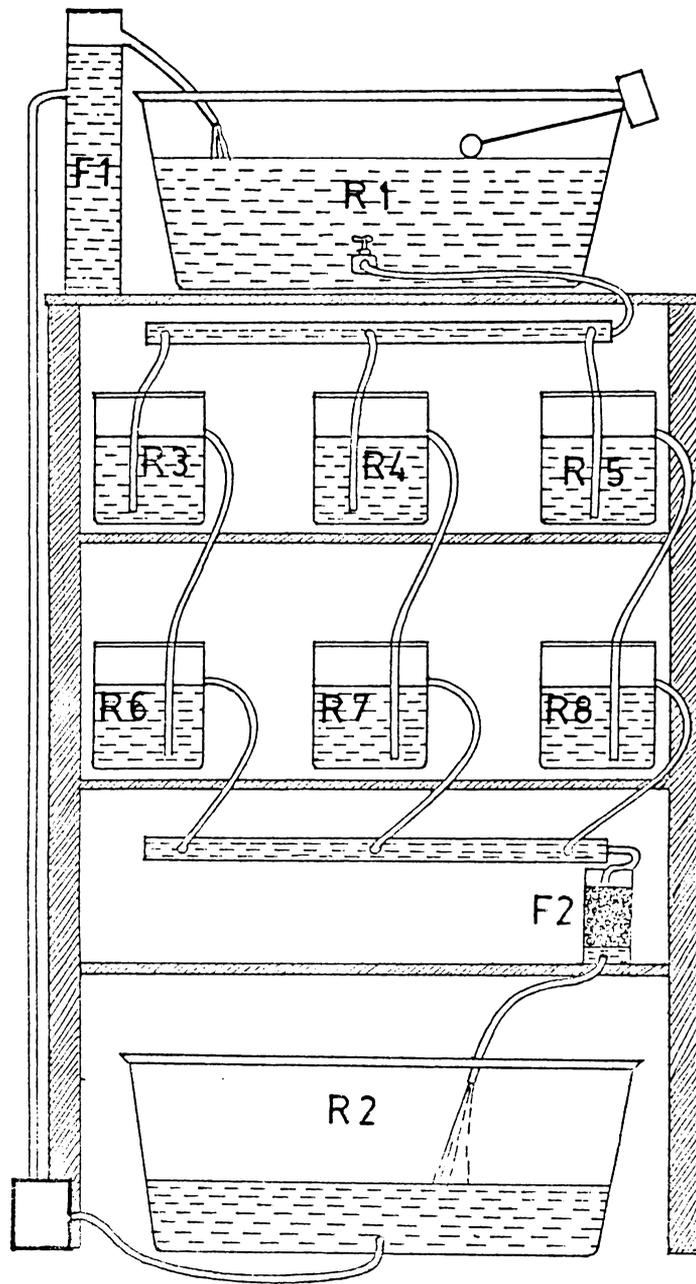
R<sub>1</sub>-Upper reservoir      F<sub>1</sub>-Foaming tower
