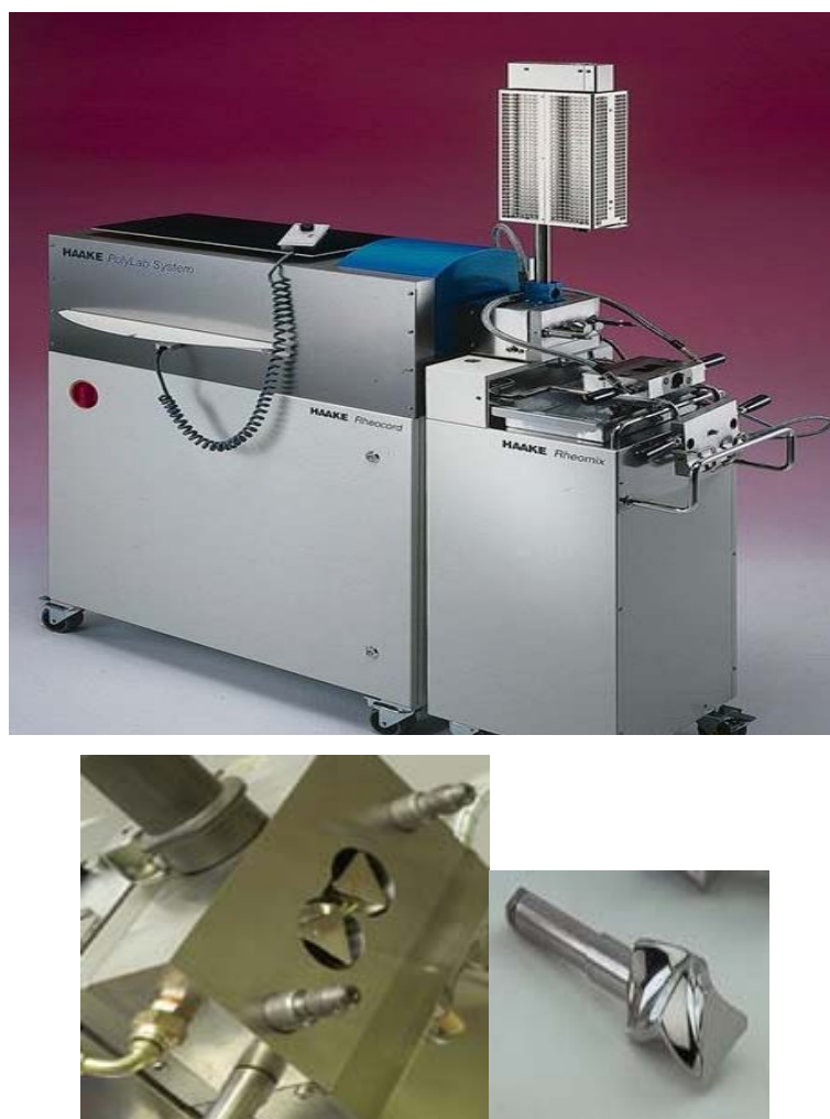
Figure 2.1 Thermo HAAKE polylab system. (Mixing chamber and the rotors are also shown)
