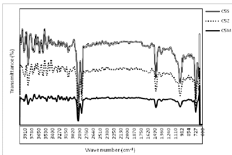
Figure 4.8 FTIR spectra of LDPE-starch-compatible blends
