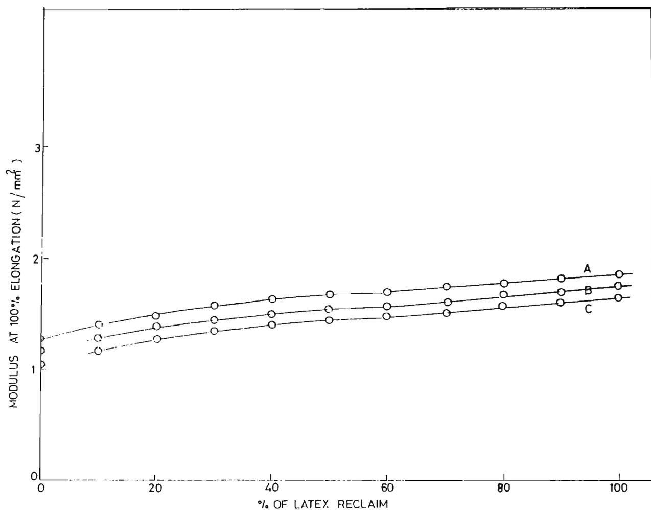
FIG.3.6: Variation in modulus with latex reclaim of NR/LR blends
