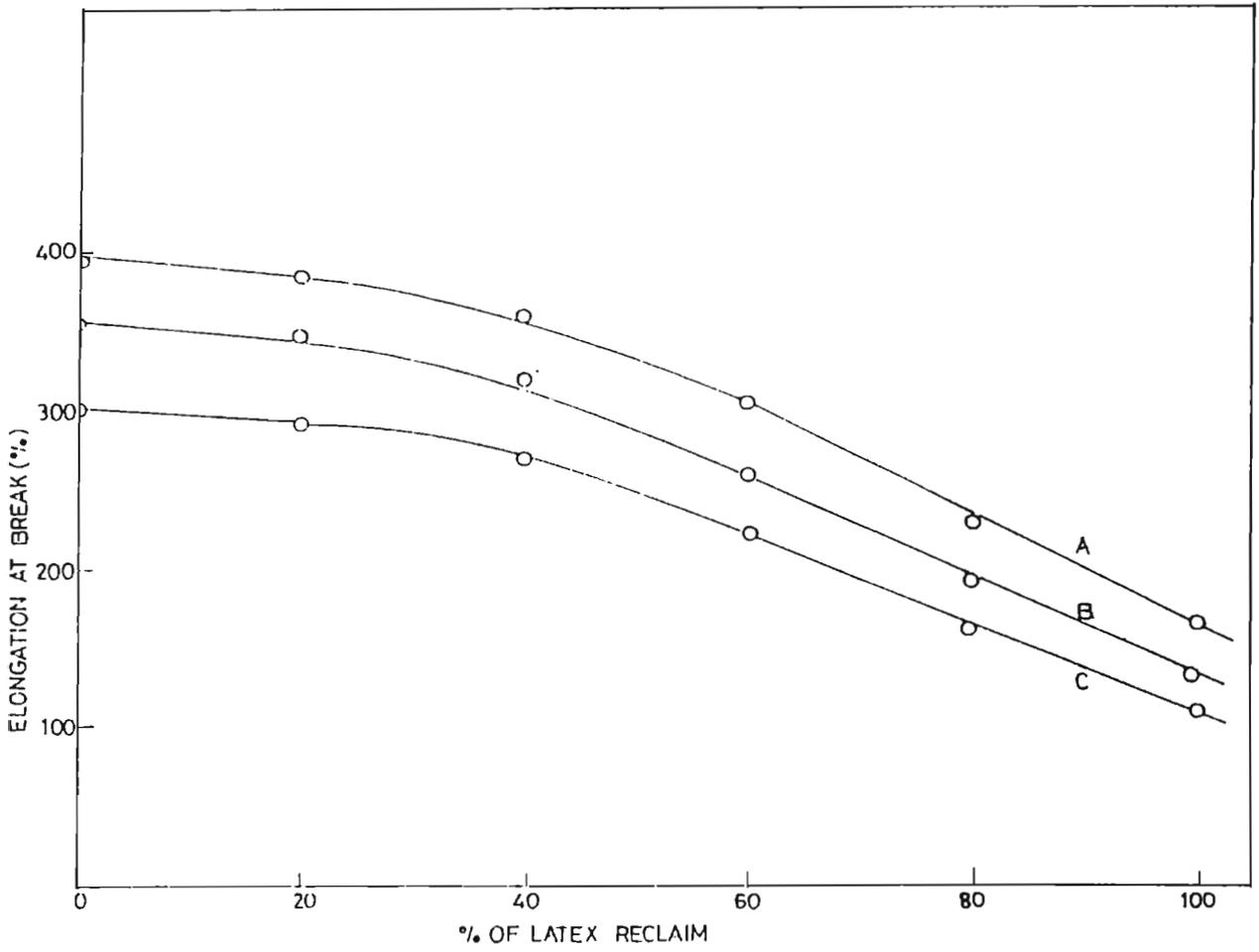
FIG.4.7: Variation in elongation at break with latex reclaim in SBR/LR blends
