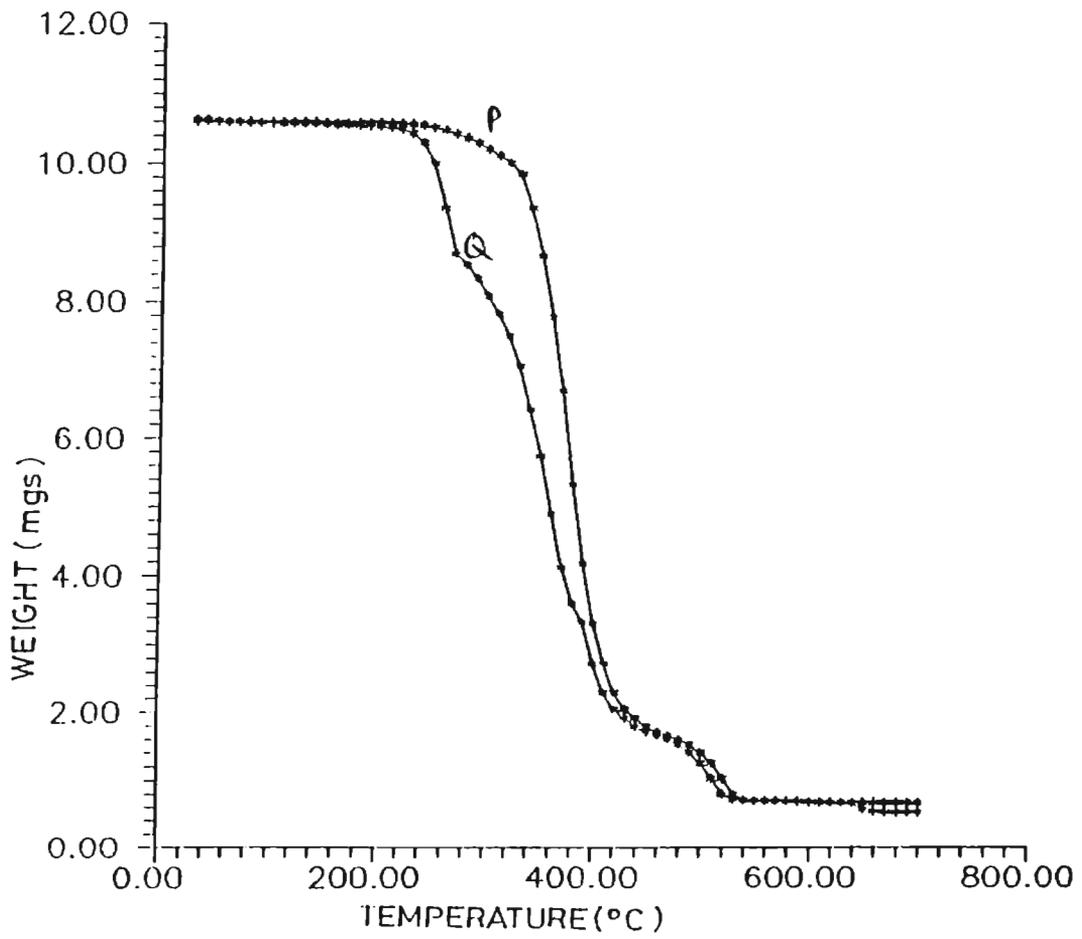
Fig.3.1: TGA graph of waste latex product (P) and latex reclaim from the final Process (Q).
