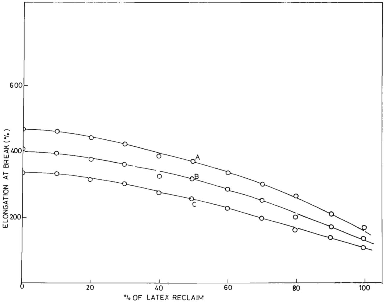
FIG.3.32: Variation in elongation at break with latex reclaim of NR/LR blends
