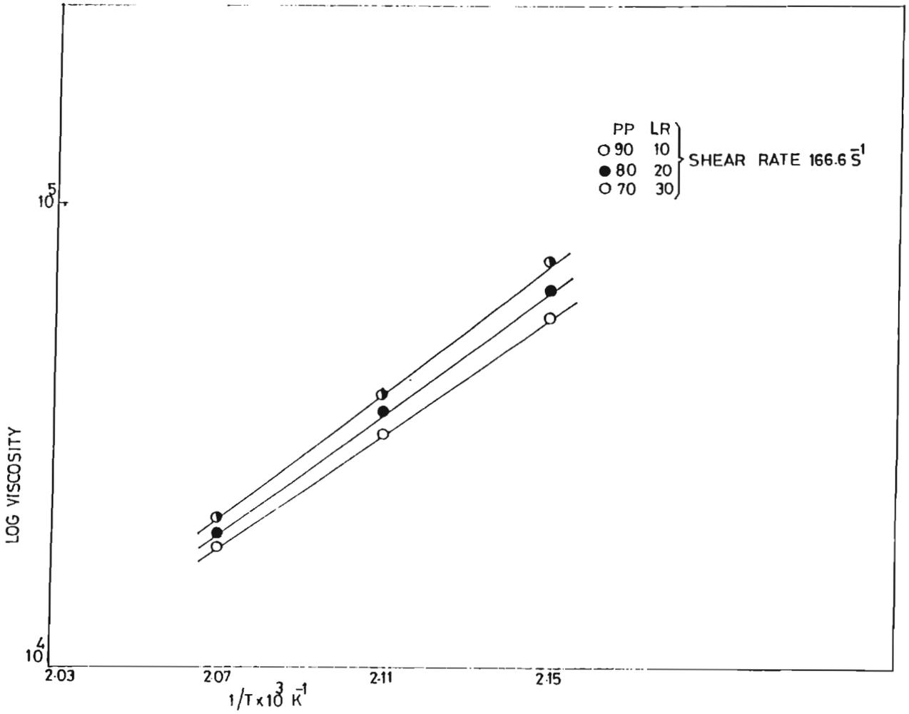
FIG.5.14: Variation in viscosity with temperature of PP/LR blends at a shear rate of  $166.6 \text{ S}^{-1}$
