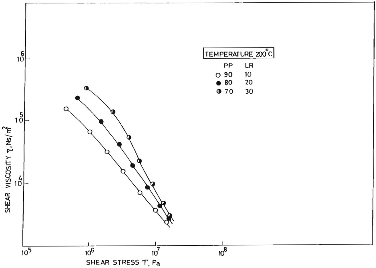
FIG.5.12: Variation in shear viscosity with shear stress of PP/LR blends at 200°C
