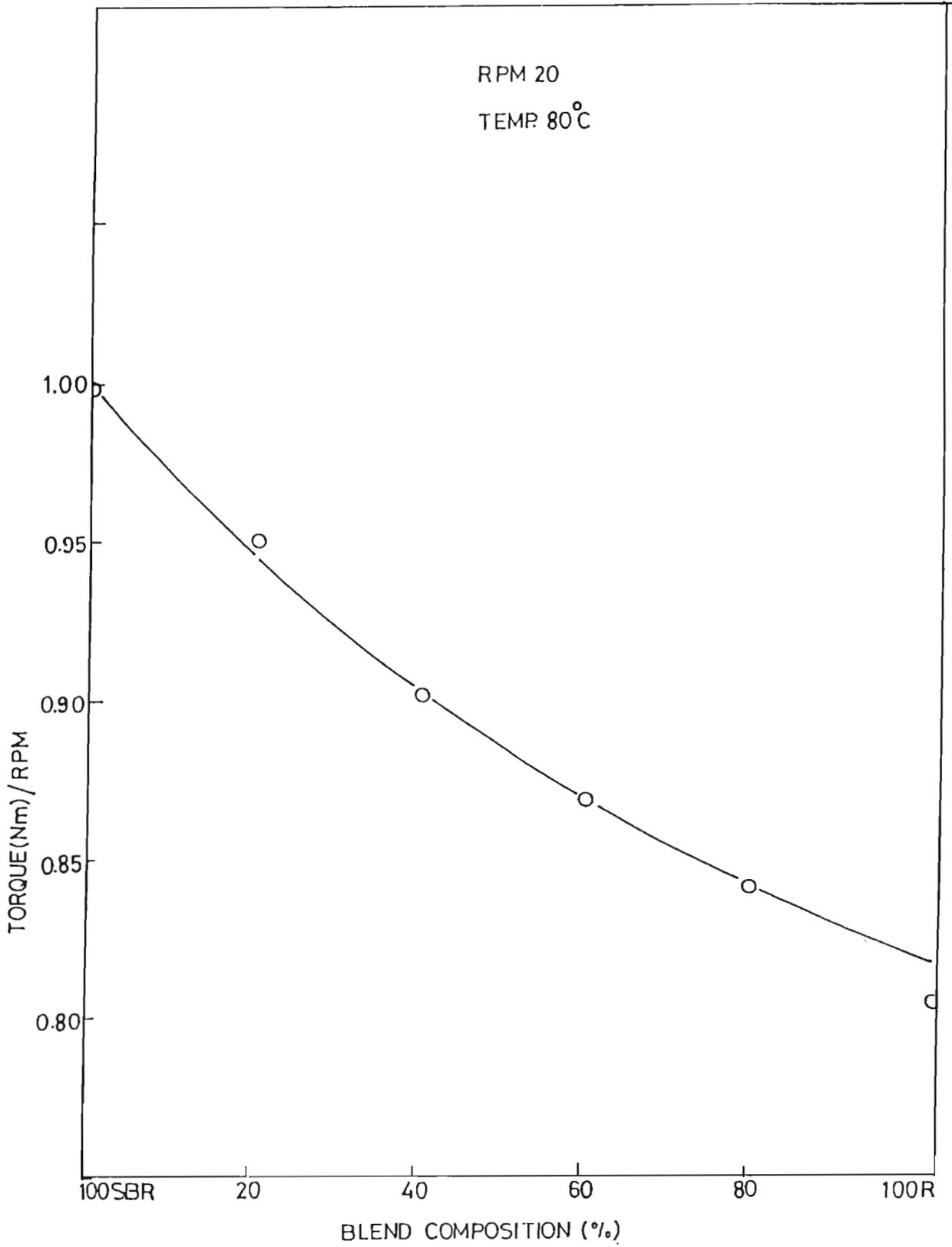
FIG.4.11: Variation in viscosity with latex reclaim of SBR/LR blends
