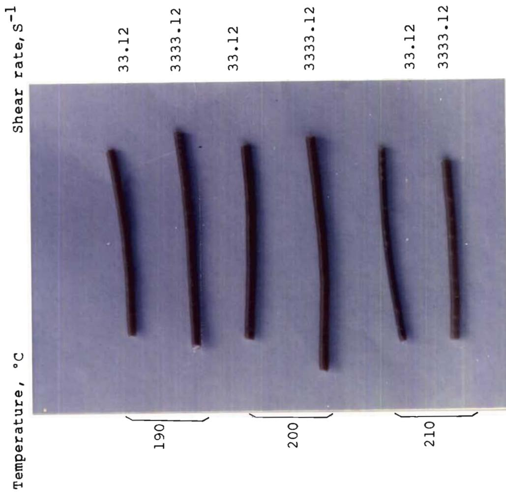
FIG. 5.17: Photograph of the extrudates of PP/LR (70/30) blend at two shear rates at different temperatures
