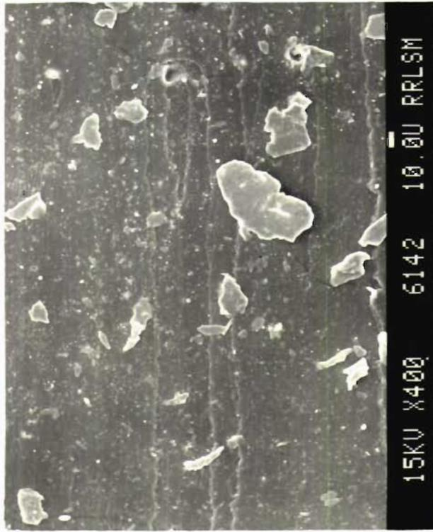
FIG.3.16: SEM photograph of the tear fracture surface of gum LR vulcanizate
