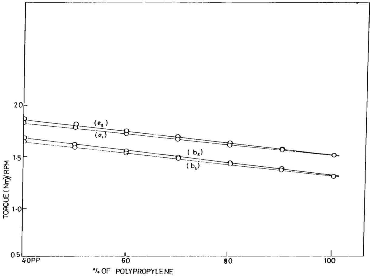
FIG.5.5: Variation in viscosity with polypropylene of uncrosslinked  $b_1$  (PP/NR);  $b_2$  (PP/LR) and crosslinked  $e_1$  (PP/NR);  $e_2$  (PP/LR) blends
