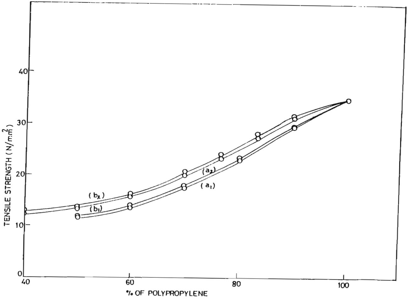
FIG.5.1: Variation in tensile strength with polypropylene of uncrosslinked  $a_1, b_1$  (PP/NR);  $a_2, b_2$  (PP/LR) blends
