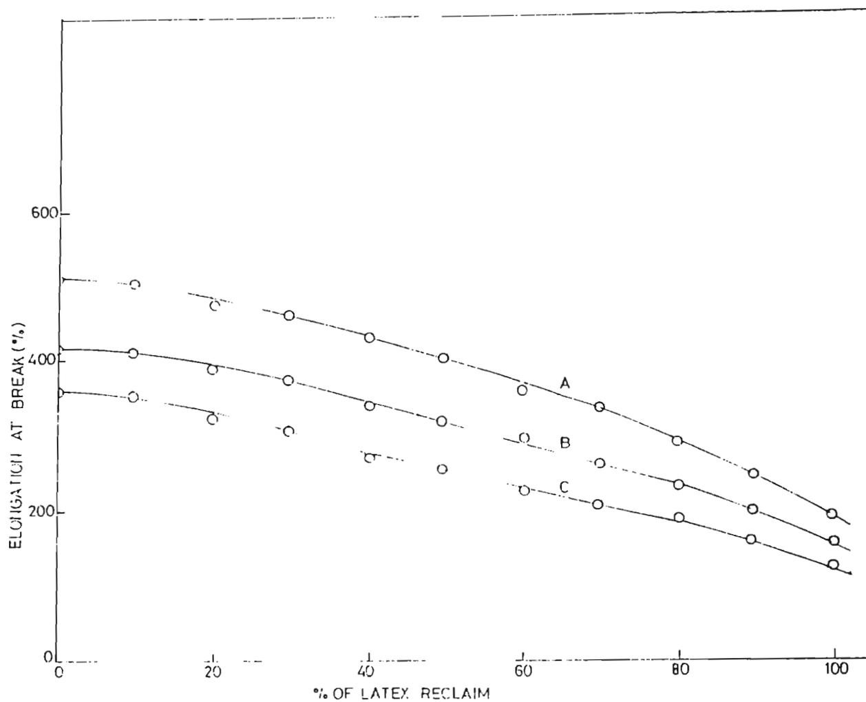
FIG.3.5: Variation in elongation at break with latex reclaim of NR/LR blends
