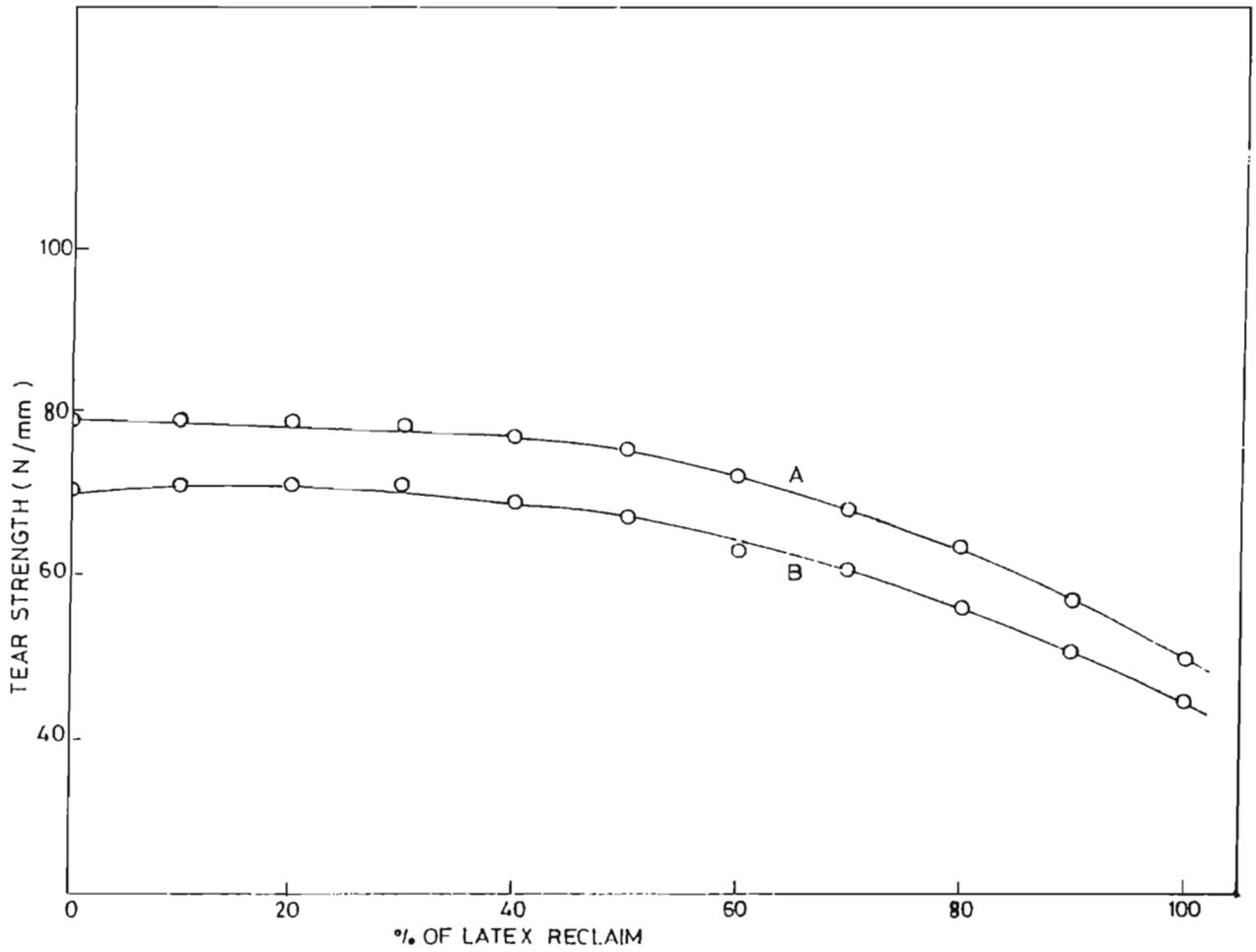
FIG.3.31: Variation in tear strength with latex reclaim of NR/LR blends
