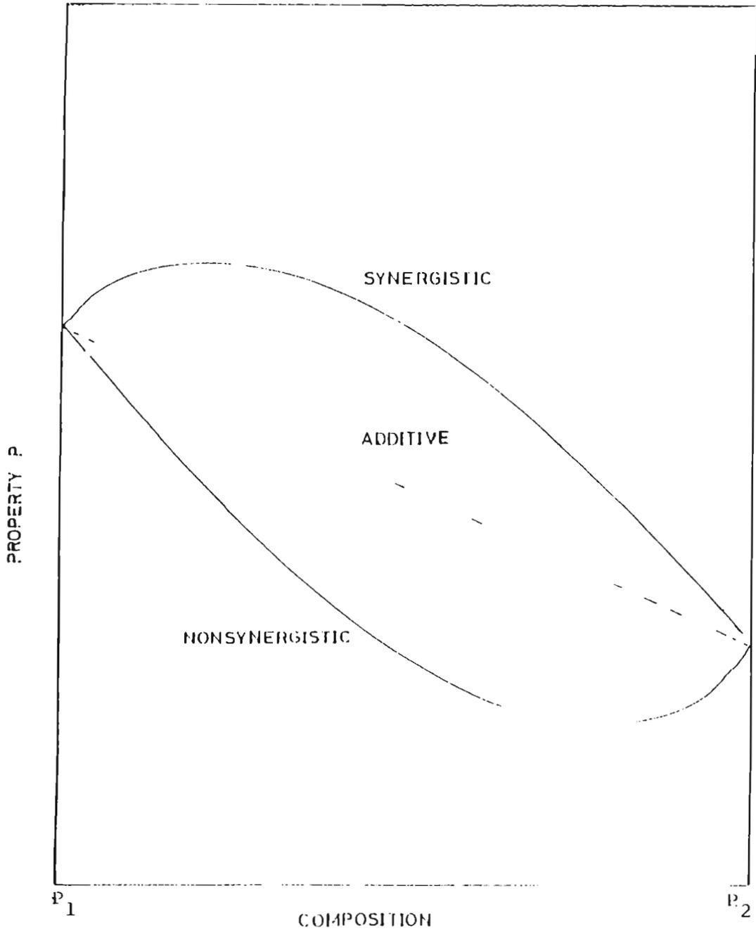
Fig.1.1: Variation of property with composition for a binary polymer blend
