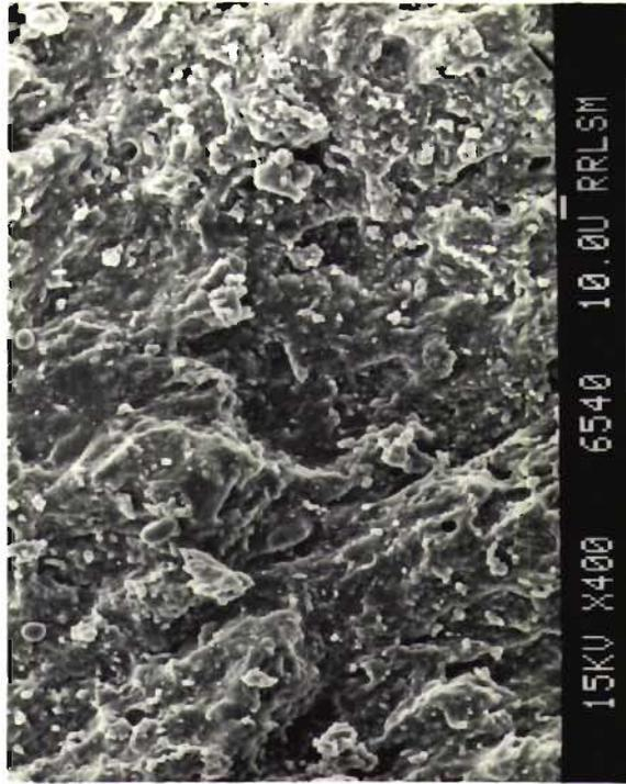
FIG.3.47: SEM photograph of the abraded surface of filled LR vulcanizate
