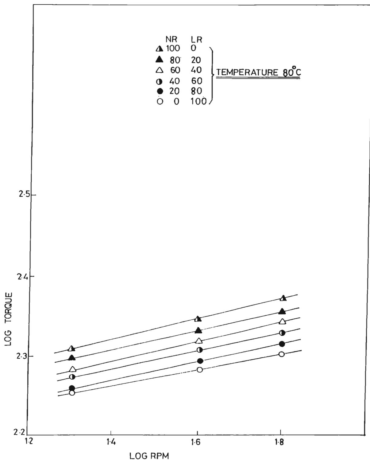
FIG.3.49: Variation in torque with shear rate of NR/LR blends at 80°C
