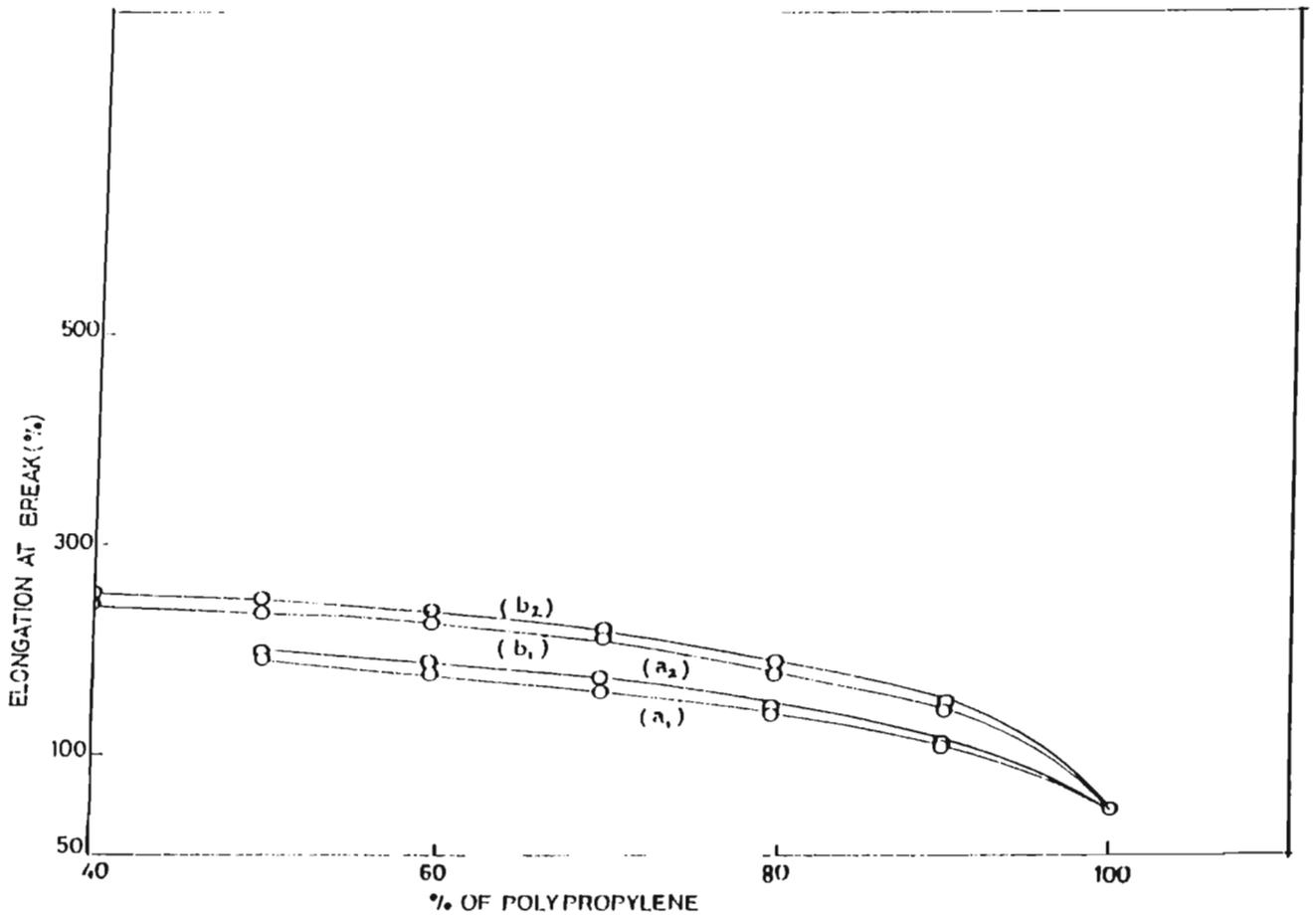
FIG.5.3: Variation in elongation at break with polypropylene of uncrosslinked  $a_1, b_1$  (PP/NR);  $a_2, b_2$  (PP/LR) blends
