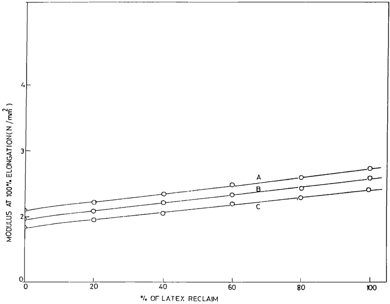
FIG.4.6: Variation in modulus with latex reclaim of SBR/LR blends
