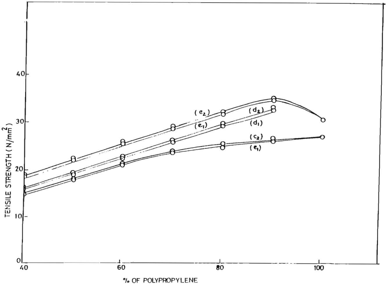
FIG.5.2: Variation in tensile strength with polypropylene of crosslinked  $c_1, d_1, e_1$  (PP/NR);  $c_2, d_2, e_2$  (PP/LR) blends
