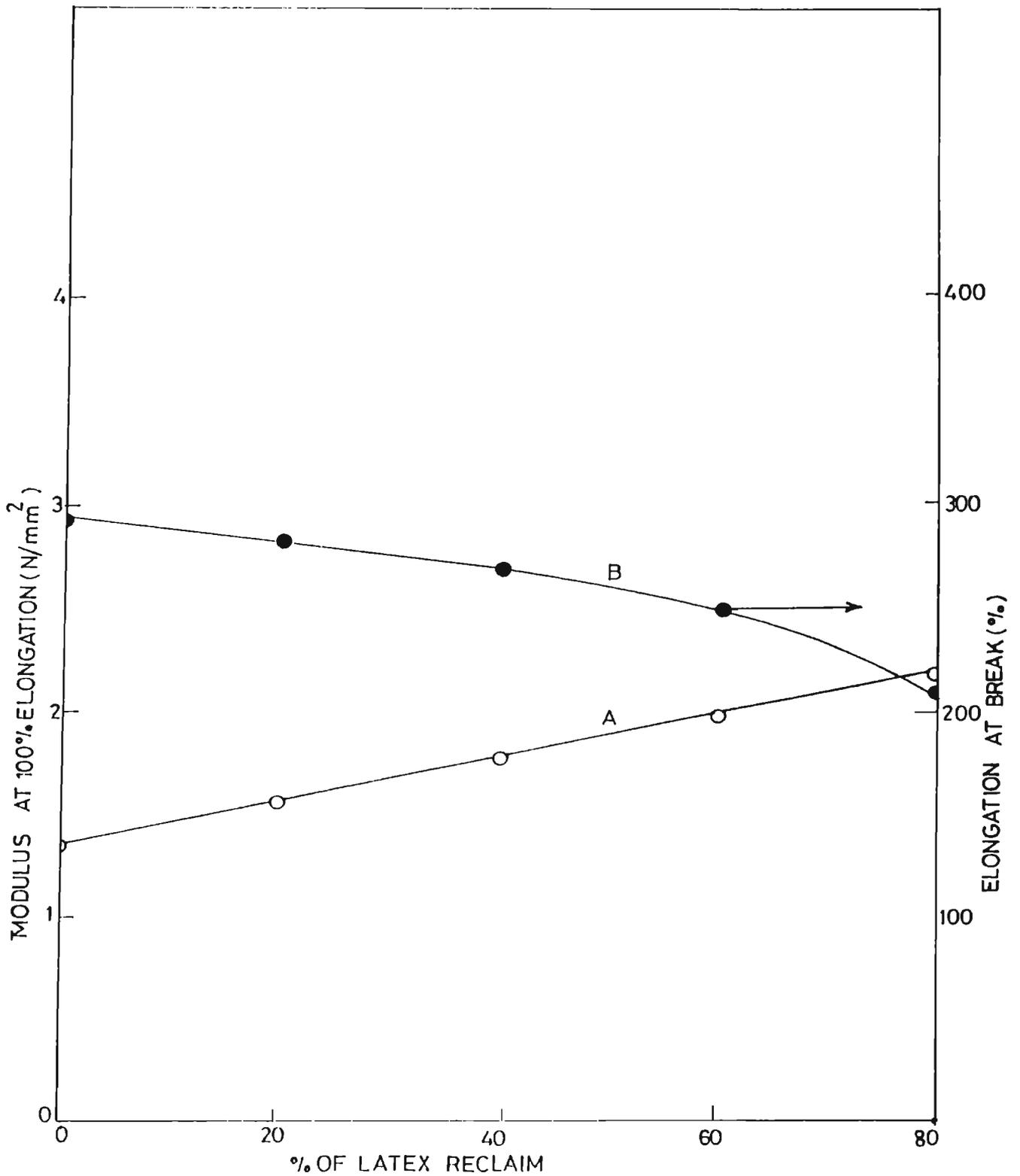
FIG.4.2: Variation in modulus and elongation at break with latex reclaim of SBR/LR blends
