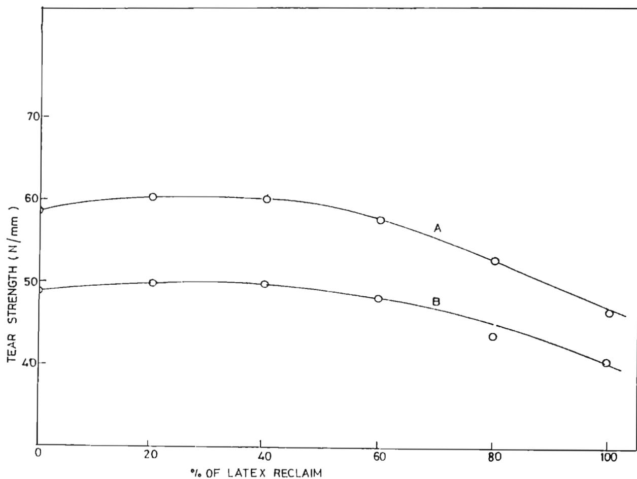
FIG.4.5: Variation in tear strength with latex reclaim of SBR/LR blends
