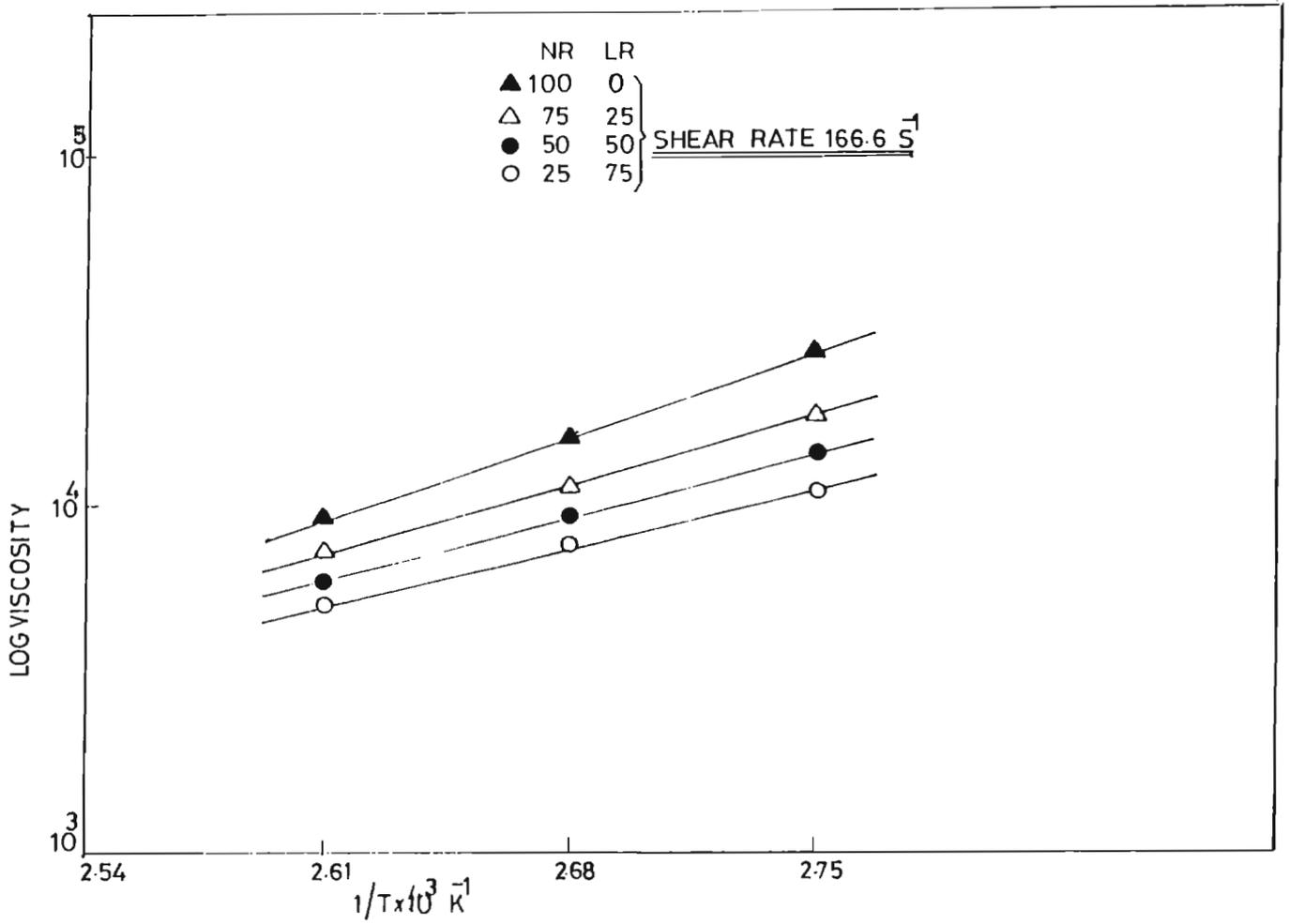
FIG.3.53: Variation in viscosity with temperature of NR/LR blends at a shear rate of  $166.6 \text{ S}^{-1}$
