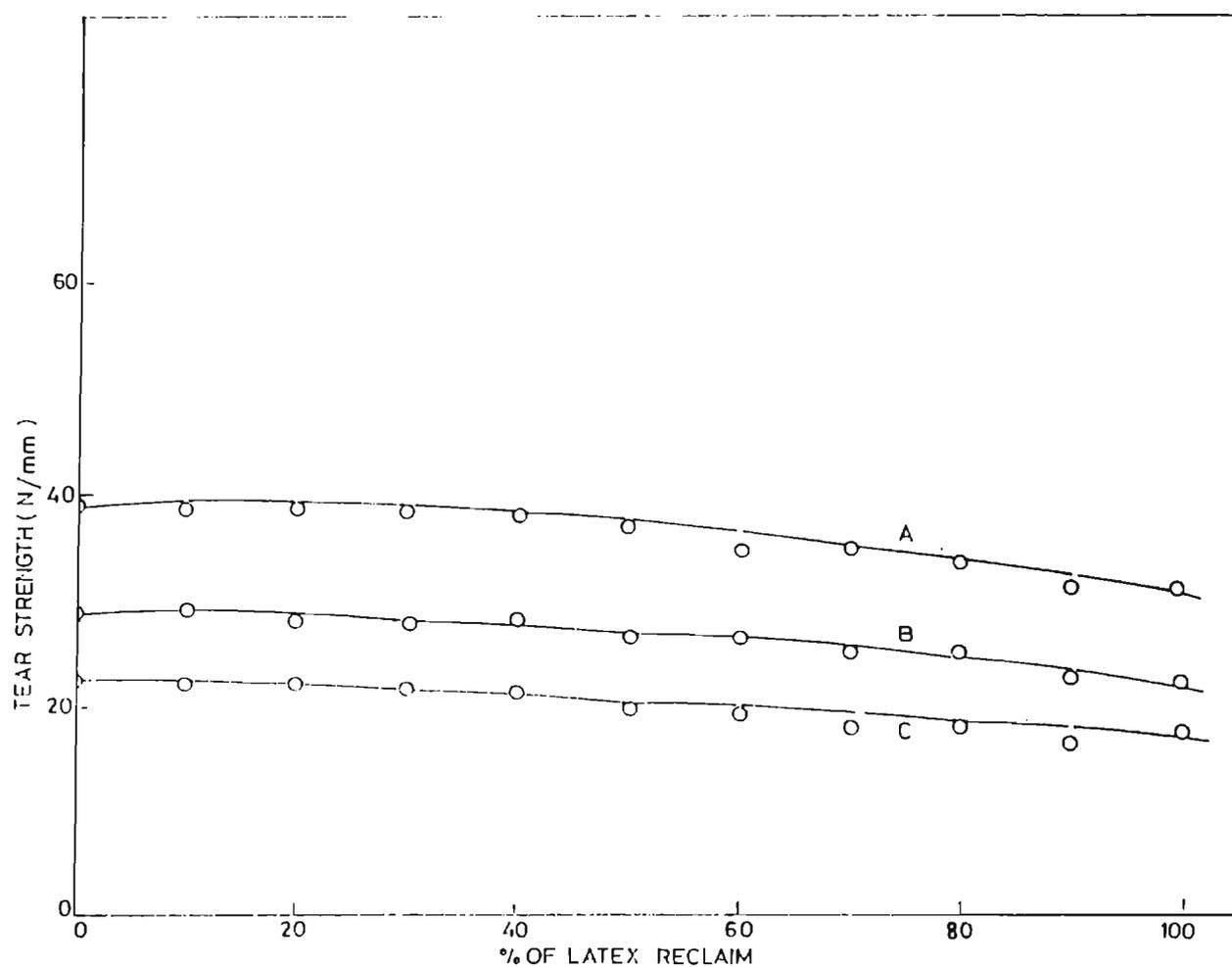
FIG.3.4: Variation in tear strength with latex reclaim of NR/LR blends
