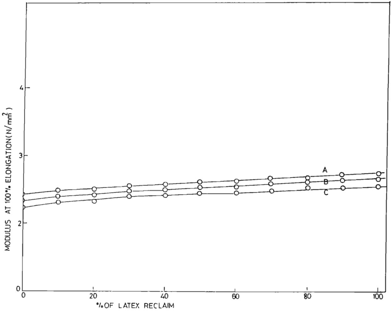
FIG.3.33: Variation in modulus with latex reclaim of NR/LR blends
