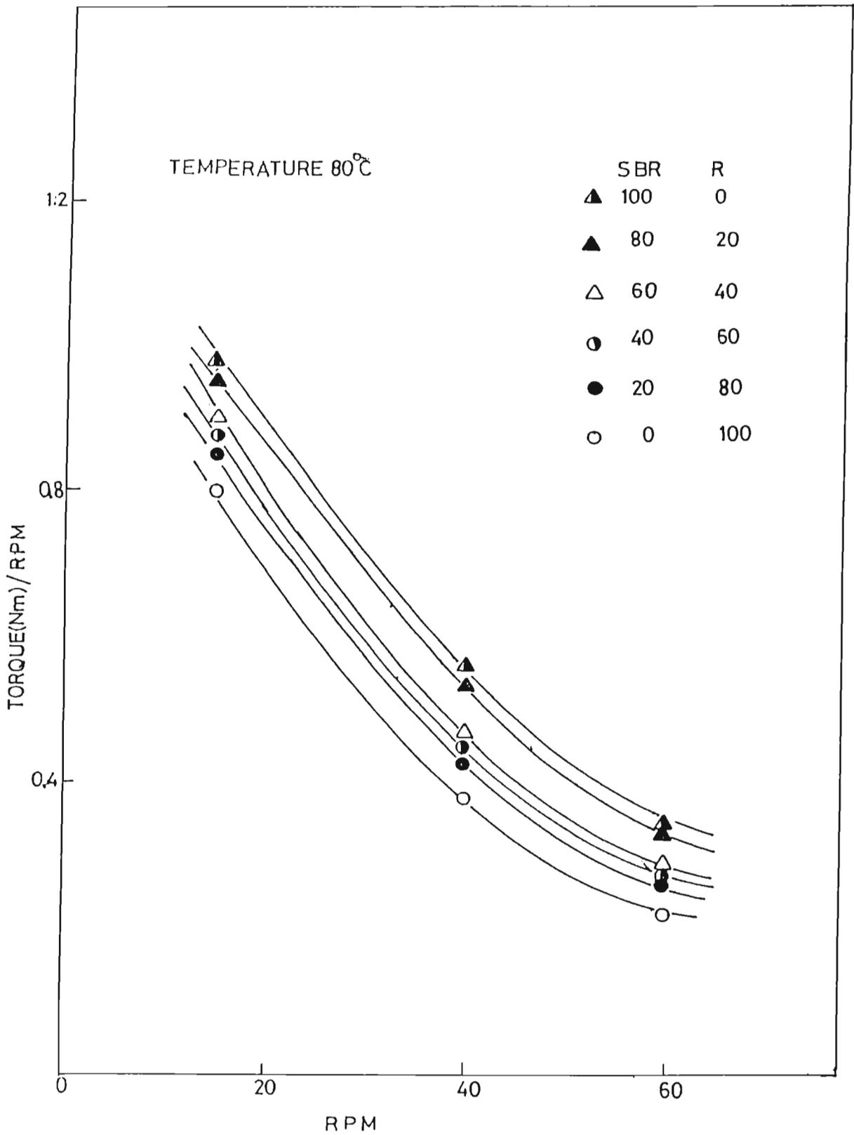
FIG.4.8: Variation in viscosity with shear rate of SBR/LR blends at 80°C
