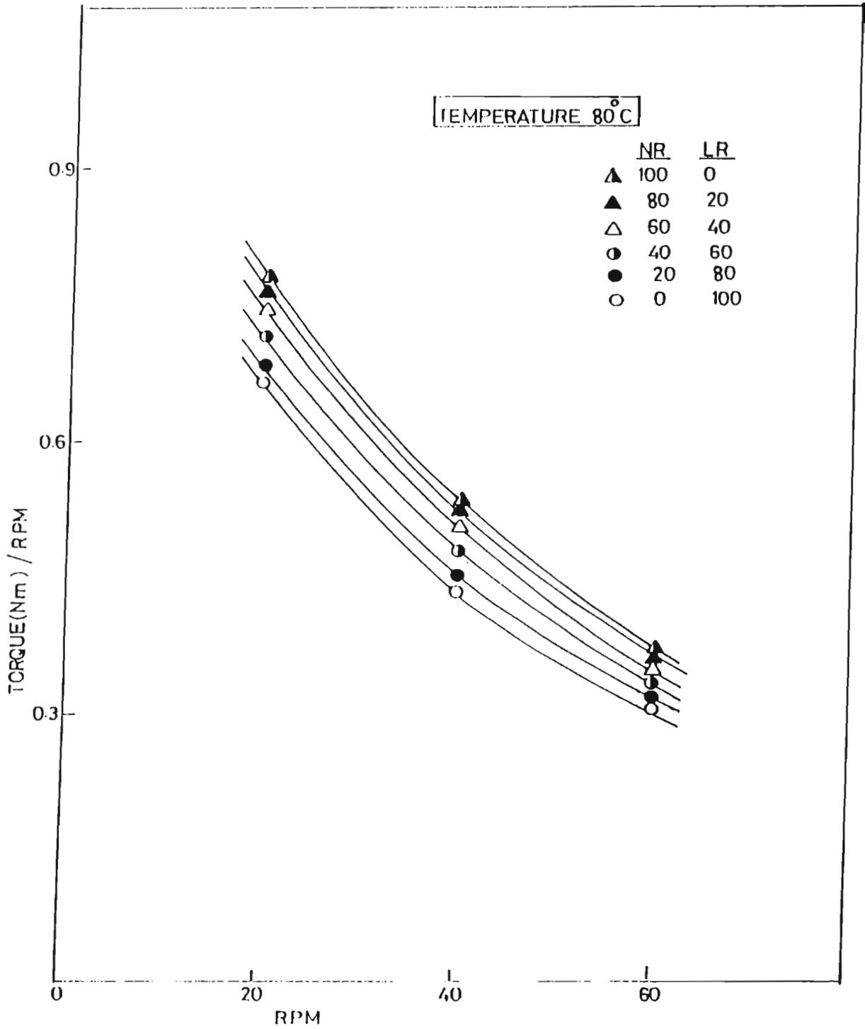
FIG.3.27: Variation in viscosity with shear rate of NR/LR blends at 80°C
