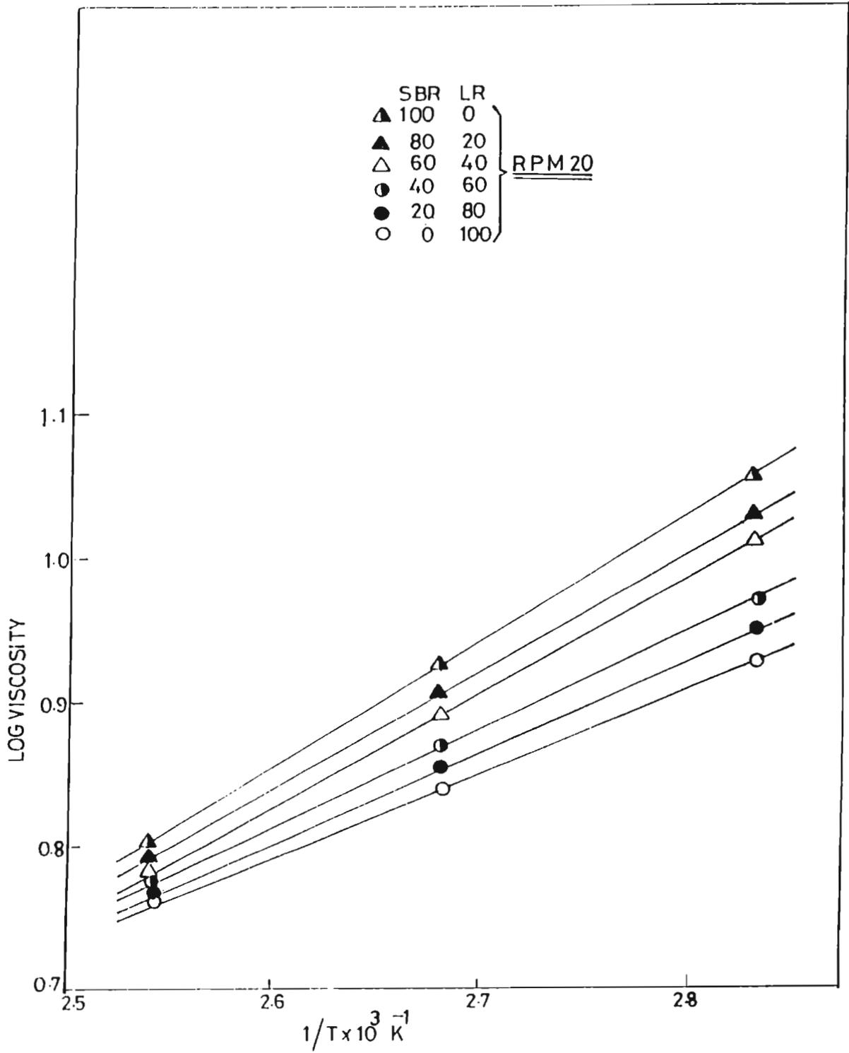
FIG.4.10: Variation in viscosity with temperature of SBR/LR blends at 20 rpm
