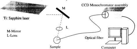
Figure 3.17: Schematic representation of the experimental arrangement for frequency upconversion studies.
