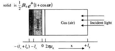
Figure 1.12: cross sectional view of a simple cylindrical photoacoustic cell (PAC).
