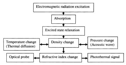
Figure 1.11: Basic processes responsible for photothermal (PT) signal generation.
