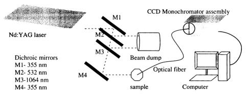
Figure 3.5: Schematic diagram of the experimental setup for measuring the photoluminescence (PL) of rare earth titanates (RETs).
