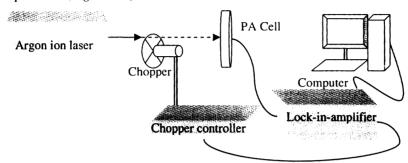
Figure 3.22: Schematic representation of photoacoustic (PA) experimental setup.
