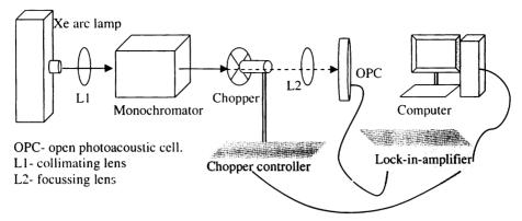
Figure 3.14: Schematic representation of photoacoustic spectroscopy experimental setup.
