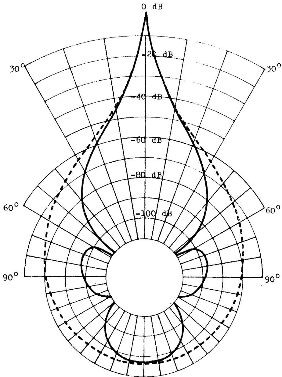
Fig.5.2 : Directivity patterns with and without the aperture term for 15 kHz difference frequency signal
