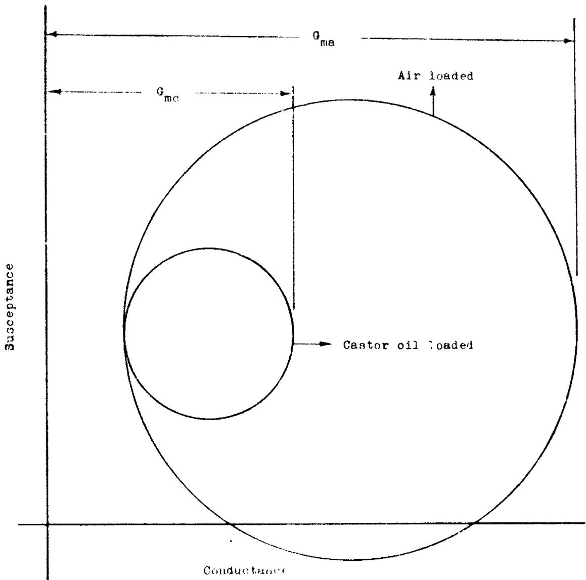
Fig.6.7 : Admittance diagram of ceramic transducer elements with air and castor oil loadings
