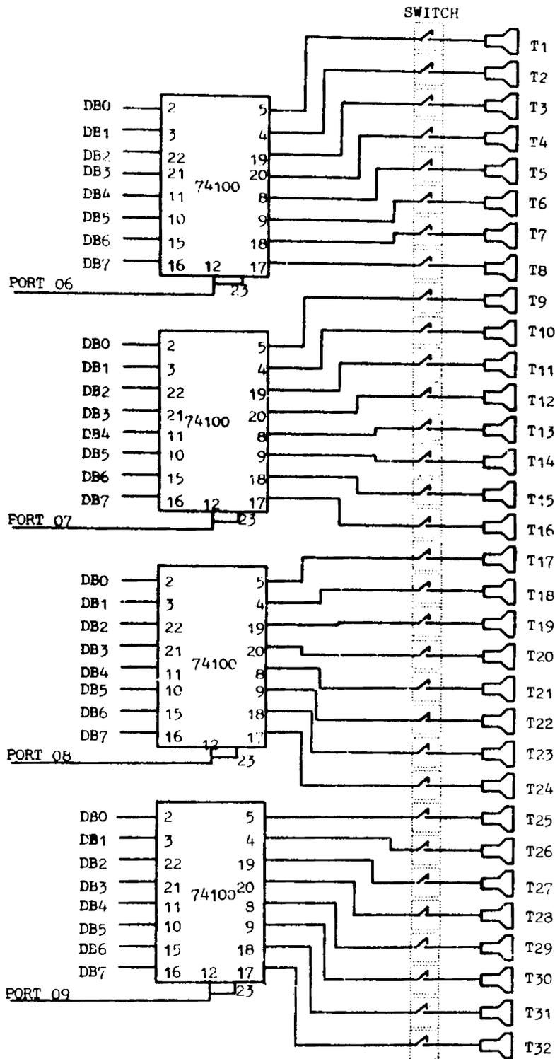
Fig.A.II.1: LATCHING UNIT OF THE SWITCHING SYSTEM
