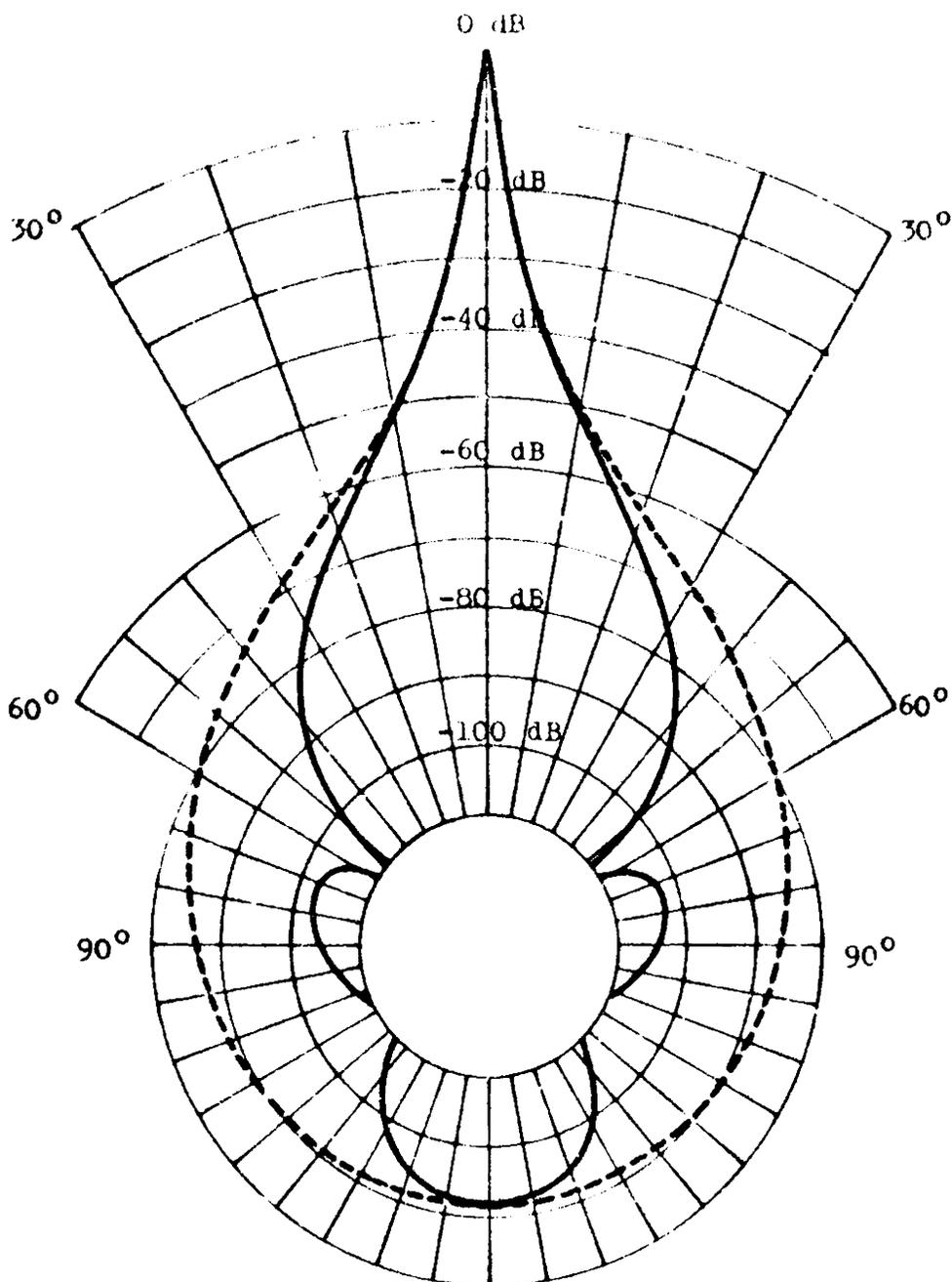
Fig.5.1 : Directivity patterns with and without the aperture term for 3 kHz difference frequency signal (Full line and dotted line drawings, respectively represent the patterns with and without the aperture term)
