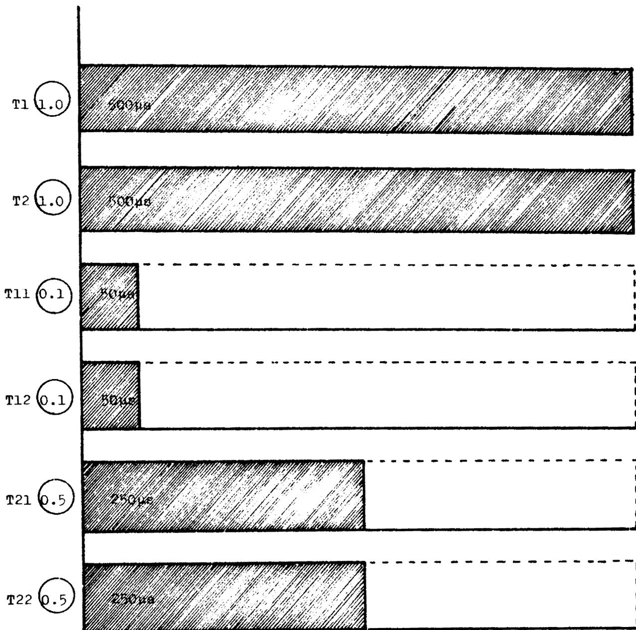
Fig.A.IV.1 : Output switching time durations for different elements of a 6-element linear array for the Binomial Shading
