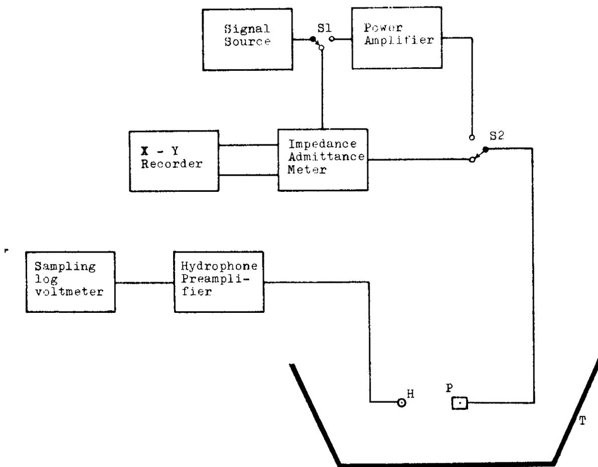
Fig.6.6 : Experimental set-up for investigating the effect of depth of immersion on the efficiency of radiation of a ceramic transducer element
