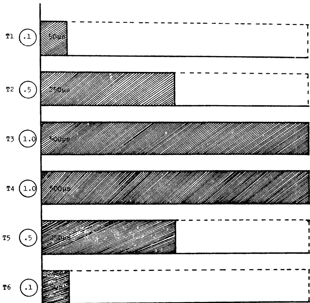
Fig.4.1 : Illustration of the output switching time durations for different elements of a 6-element linear array for the Binomial Shading
