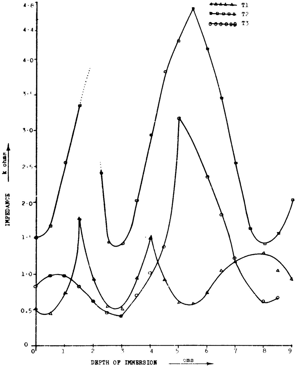
Fig.6.3: Variation of impedance at resonance of ceramic transducer elements with depth of immersion of the radiating face
