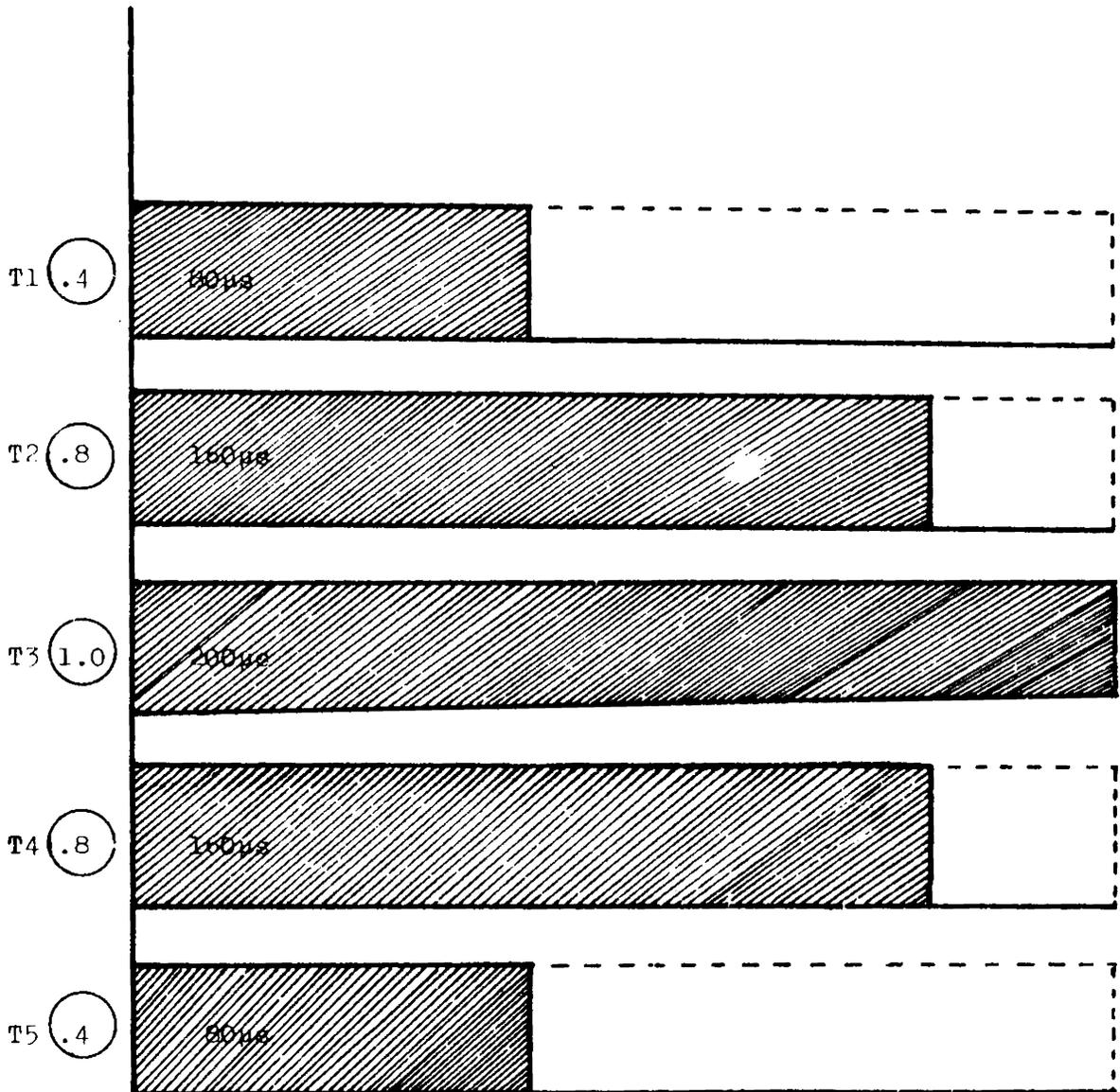
Fig.4.3 : Illustration of the output switching time durations for various elements of a 5-element linear array for the continuous Distribution Shading
