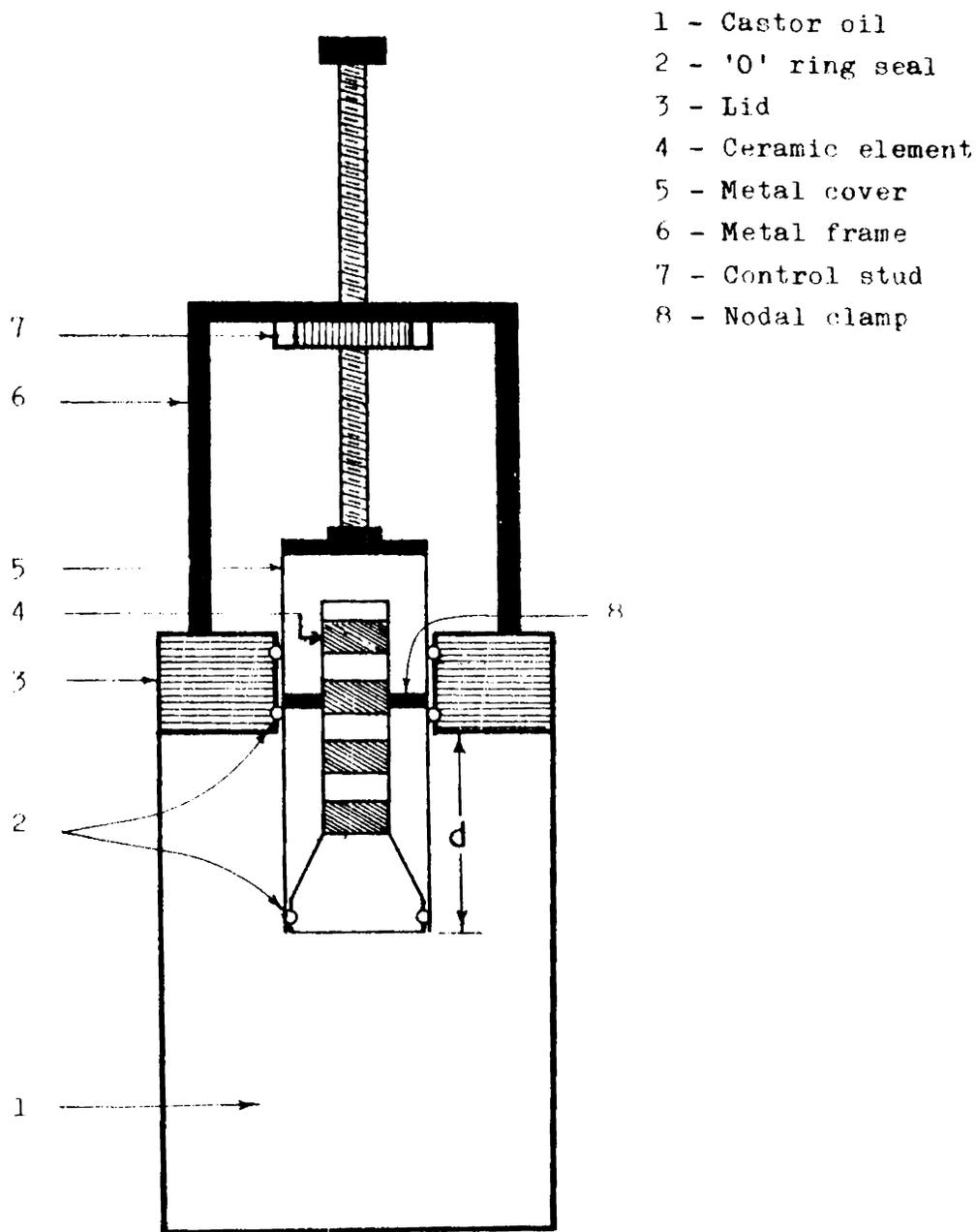
Fig.6.1 : Set-up of the projector assembly, used to investigate the effect of finite medium
