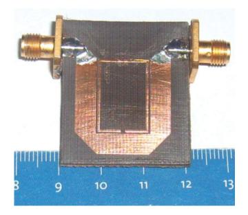
**Figure 2** Photograph of OLRR filter. [Color figure can be viewed in the online issue, which is available at www.interscience.wiley.com]
