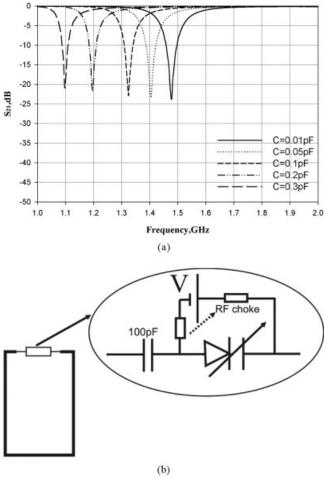
**Figure 4** (a) Simulated results of notch frequency tuning of the OLRR filter (b) DC isolation circuit for connecting the varactor
