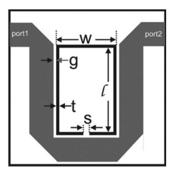
**Figure 1** Geometry of the proposed OLRR narrow band reject filter (l = 17 mm, w = 12 mm, s = 1 mm, t = 0.5 mm)
