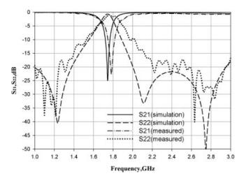
Figure 3 Transmission characteristics of the OLRR filter
