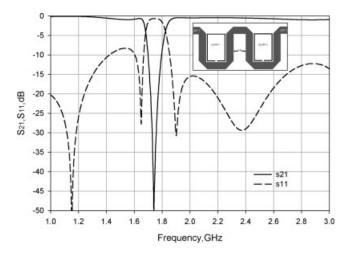
Figure 5 Simulated response of notch filter with two OLRR elements (inset: layout)
