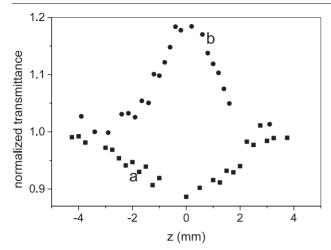
**Figure 2.** Open aperture Z-scan curve at  $532 \,\mathrm{nm}$ : (a)  $0.08 \,\mathrm{J\,cm^{-2}}$ ; (b)  $0.5 \,\mathrm{J\,cm^{-2}}$ .
