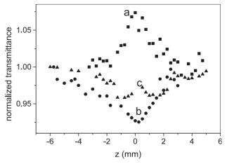
**Figure 4.** Open aperture Z-scan curve at 456 nm: (a)  $0.1 \,\mathrm{J\,cm^{-2}}$ ; (b)  $0.2 \,\mathrm{J\,cm^{-2}}$ ; (c)  $0.6 \,\mathrm{J\,cm^{-2}}$ .
