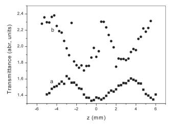
**Figure 3.** Open aperture Z-scan curve at 477 nm: (a)  $0.08 \,\mathrm{J\,cm^{-2}}$ ; (b)  $0.44 \,\mathrm{J\,cm^{-2}}$ .
