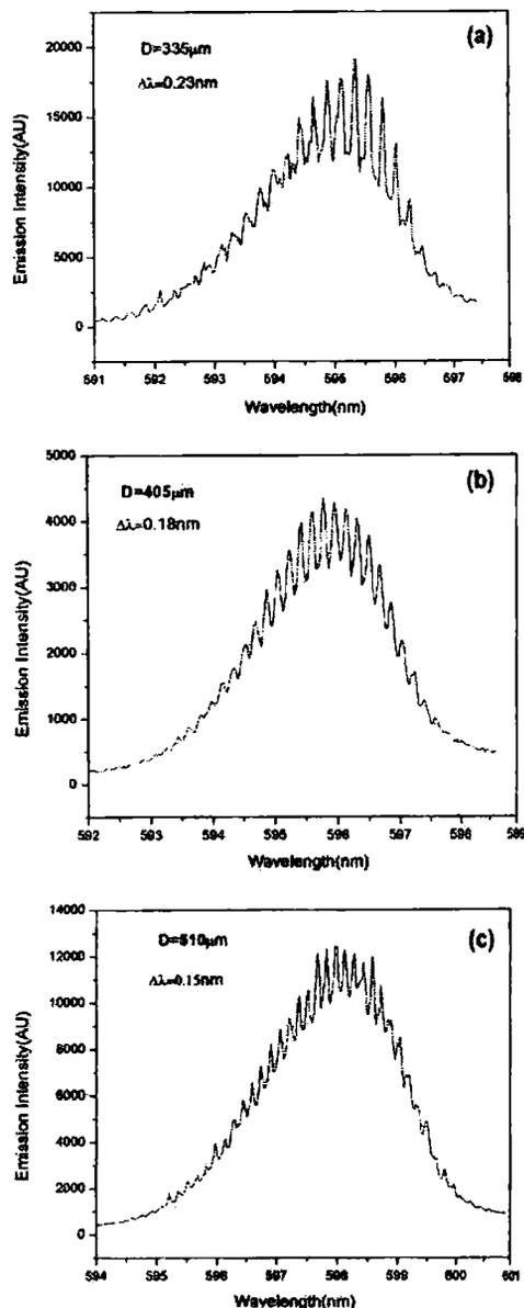
Fig. 6. Multimode laser emission from 7 cm long dye doped fiber at a pump energy 1.37 mJ/pulse.  $D$  = (a) 335, (b) 405, and (c) 510  $\mu\text{m}$ .
