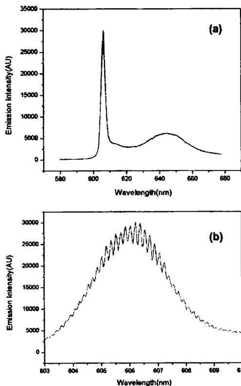
Fig. 5. (a) Typical multimode laser emission spectrum at a pump energy of 0.47 mJ/pulse from a POF doped with equal concentrations (0.25 mM) of Rh 6G and Rh B. (b) Expanded modes in (a).
