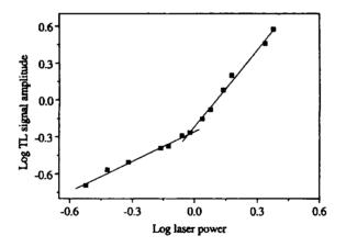
Fig. 4. Log-log plot of thermal lens signal amplitude against laser power.
