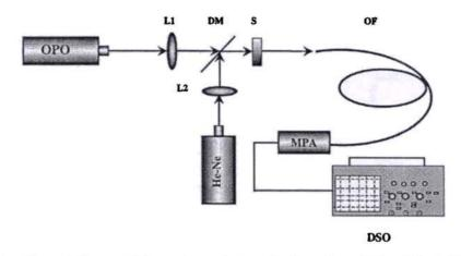
Fig. 1. Schematic diagram of the experimental set up.  $L_1$ ,  $L_2$  – Lens; DM – Dichoric Mirror; S – Sample; OF – Optic Fibre; MPA-Monochromator – PMT assembly; DSO – Digital Storage Oscilloscope.
