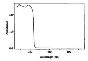
Fig. 2. The absorption spectrum of aniline.
