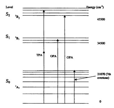
Fig. 5. Schematic energy level diagram showing relevant two-photon and one photon absorptions (TPA, OPA) along with the overtone absorption in the case of Aniline. The level  $S_2$  acquires the symmetry character of  $S_0$  by vibronic coupling so that both OP and TP absorptions are possible.
