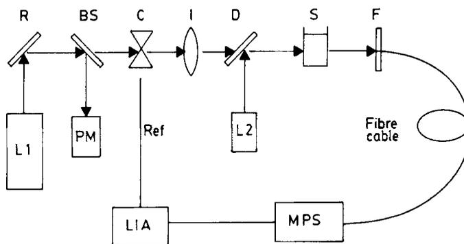
**Figure 1.** Schematic diagram of the experimental set-up. (L1 – argon ion laser; PM – power meter; C – chopper; l – lens; D – dichroic mirror; S – sample cell; L2 – probe laser; F – filter; BS – beam splitter; R – reflector; LIA – lock-in amplifier; MPS – monochromator-PMT assembly).
