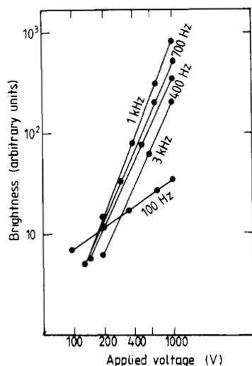
**Figure 7.** Plot of  $\log B$  against  $\log V$  for a typical ZnS:Pr,Cl EL cell excited at different frequencies.
