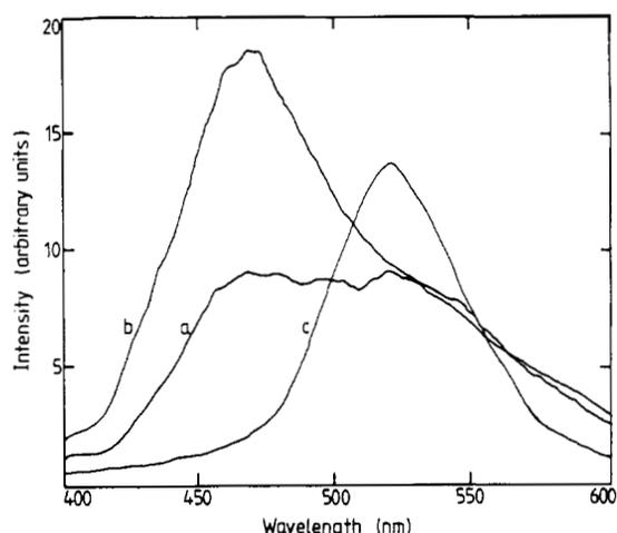
**Figure 6.** EL emission spectra of ZnS phosphors without any activators at various excitation frequencies under 400 V peak-to-peak. a, 100 Hz; b, 2.5 kHz and c, EL spectrum of ZnS:Ag,Pr,Cl (Ag 0.5 wt%, Pr 0.5 wt%) under 1 kHz excitation frequency 400 V peak-to-peak (c recorded at much reduced gain).
