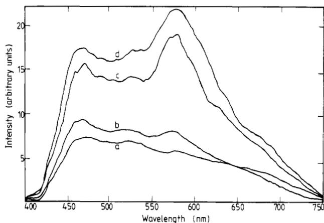
**Figure 5.** EL spectra of ZnS:Cu,Pr,Cl phosphors at 1 kHz excitation frequency. a, 400 V; b, 500 V; c, 600 V and d, 800 V peak-to-peak.
