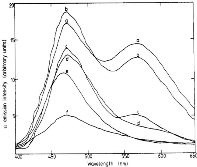
**Figure 1.** EL spectra of ZnS:Pr,Cl phosphors containing various concentrations of Pr. a, b, c, d, e and f are phosphors containing 1.0, 0.5, 0.25, 0.1, 0.02 and 0.01 wt% of Pr respectively in the pre-fired mixture under 1 kHz excitation frequency and 400 V peak-to-peak.
