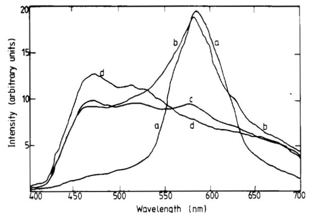
**Figure 4.** EL spectra of ZnS:Cu,Pr,Cl (Cu 0.5 and Pr 0.5 wt%) phosphors at various excitation frequencies 400 V peak-to-peak. a, 100 Hz; b, 500 Hz; c, 1 kHz and d, 2 kHz.
