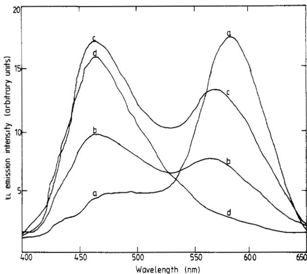
**Figure 2.** EL emission spectra of ZnS:Pr,Cl (Pr 0.5 wt%) at various excitation frequencies under 400 V peak-to-peak. a, 100 Hz; b, 400 Hz; c, 1 kHz and d, 4 kHz.
