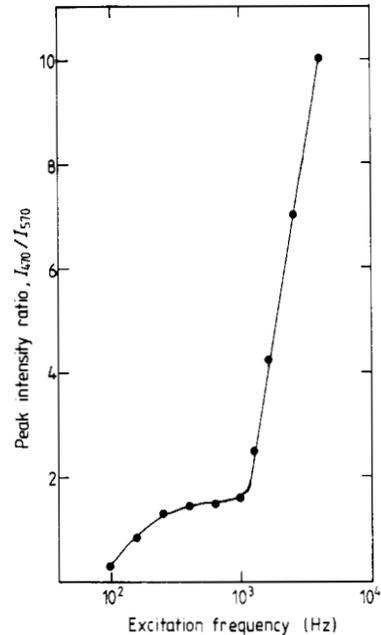
**Figure 3.** Variation of ratio of peak intensities of 470 and 570 nm bands with frequency of excitation voltage. Note that from 0.5 to 1.5 kHz the intensity remains virtually constant which is in accordance with Schön-Klasens model.
