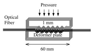
Fig. 1. Schematic diagram of the setup used to deform the optical fiber.
