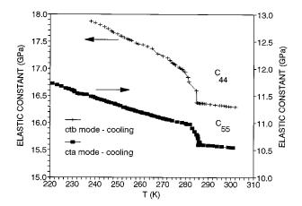
FIG. 5. Temperature variation of elastic constant for the cooling cycle of the *ctb* and *cta* modes in LAS.
