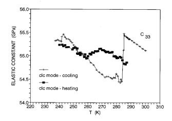
FIG. 4. Temperature variation of elastic constant for the cooling and heating cycle of the *clc* mode in LAS.
