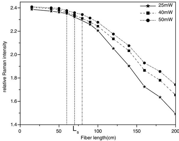
**Figure 3.** Variation of relative intensity ratio of Raman bands at 2957 and 3001  $\text{cm}^{-1}$  with fibre length.
