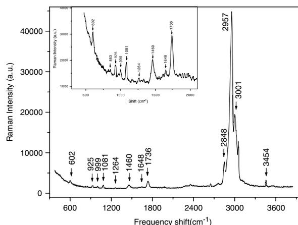
**Figure 2.** Raman spectrum of the PMMA POF pumped by 532 nm DPSS laser (50 mW). Inset shows the enhanced spectral region 500–2000 cm<sup>-1</sup>.
