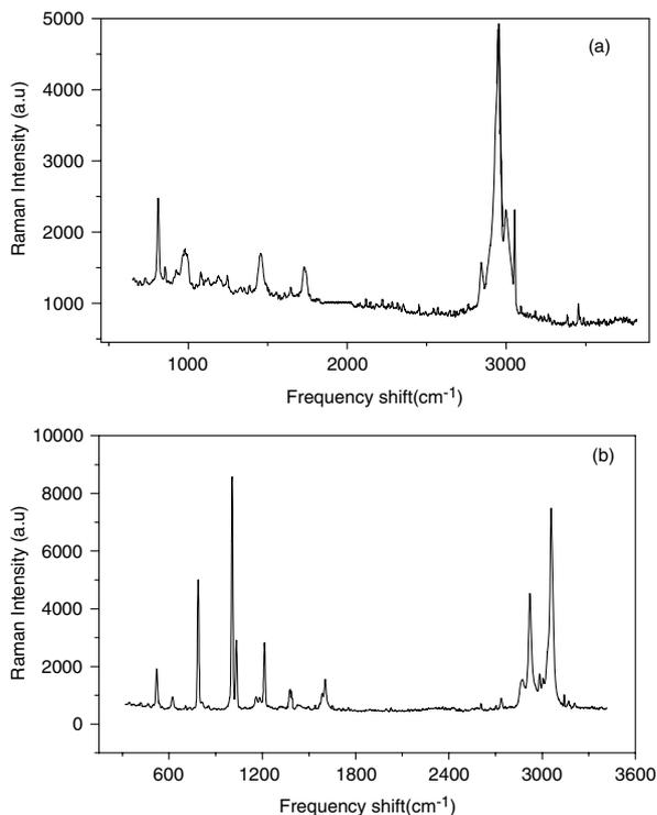
Figure 4. The Raman spectra of (a) PMMA cube and (b) toluene.
