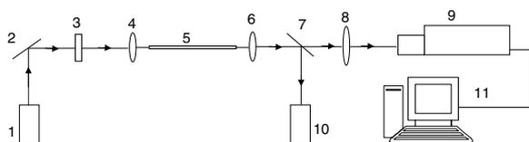
**Figure 1.** Schematic representation of the experimental set-up for measuring Raman spectrum. (1) DPSS (532 nm, cw, 50 mW); (2), (7) dichroic mirror (532 nm); (3) ND filter; (4), (6), (8) lenses; (5) PMMA POF; (9) monochromator with CCD; (10) beam dump; (11) computer for data acquisition.
