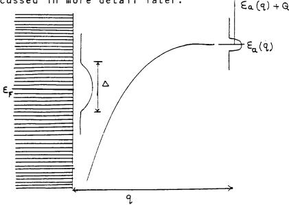
Fig.IV. The electronic energy level of the  $H_30^{\circ}$ ,  $\varepsilon_a$ , as a function of the distance from the metal, q. Q represents the shift of the ionic orbital due to the interaction with the solvent.  $\triangle$  is the width in energy of the ionic orbital.  $\varepsilon_F$  is the Fermi level of the metal.
