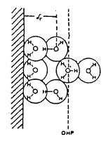
Fig.II. Bockris-Matthews model for the electrode interface in proton discharge from  $H_30^+$ .
