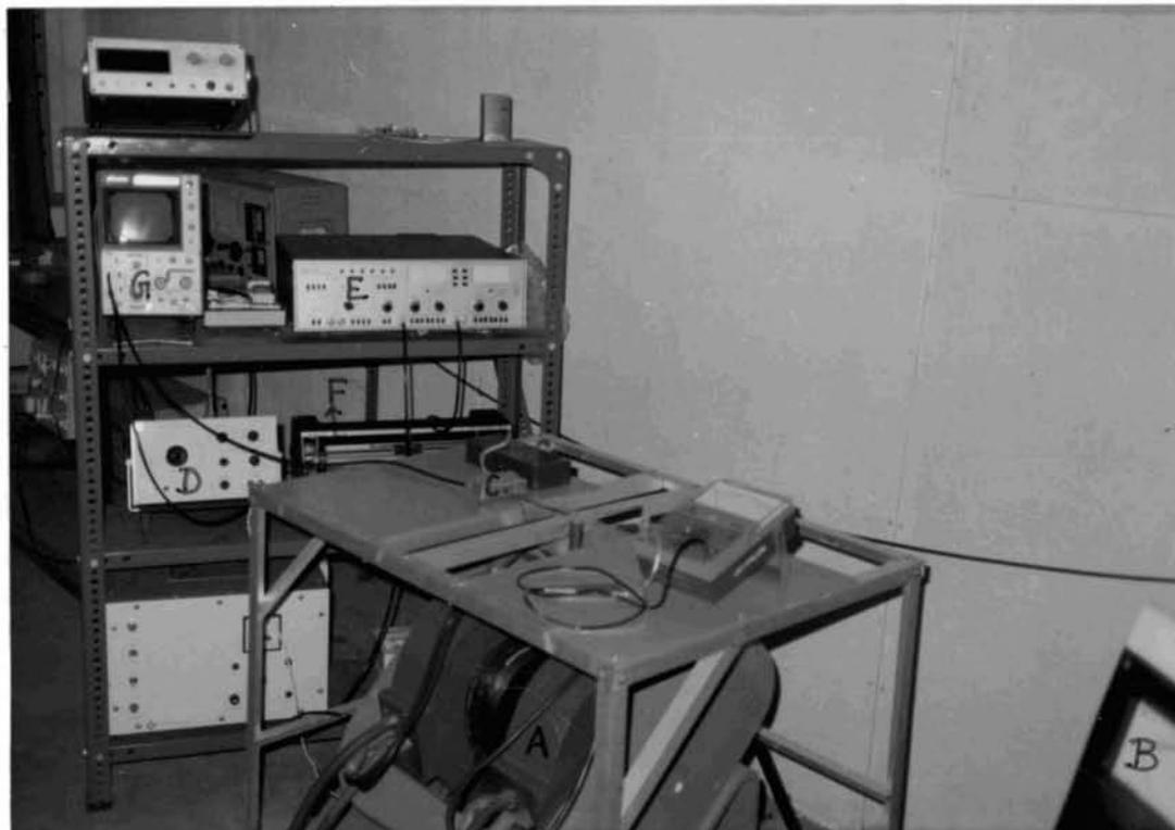
Photograph of the Wideline NMR spectrometer fabricated, showing the electromagnet (A), high current stabilizer-cum-field sweep unit (B), NMR detector (C), modulating signal generator (D), lock-in amplifier (E), chart recorder (F), C.R.O. (G) etc.
