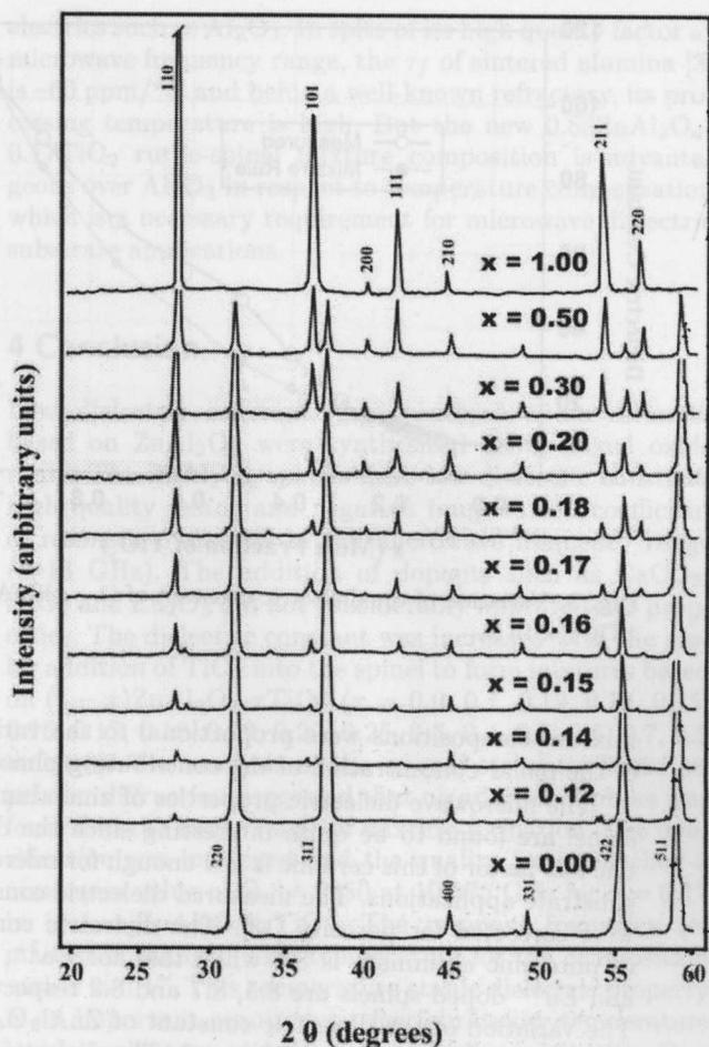
Fig. 2. Powder diffraction patterns of  $(1-x)\text{ZnAl}_2\text{O}_4-x\text{TiO}_2$  mixed phases for  $x = 0.0, 0.12, 0.14, 0.15, 0.16, 0.17, 0.18, 0.2, 0.3, 0.5, 1.0$ .
