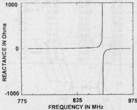
Fig. 4. Variation of input reactance with frequency for the antenna A.
