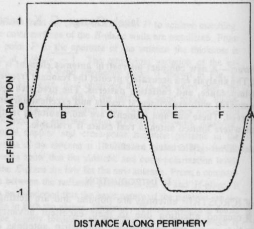
Fig. 5. Variation of normalized electric field along the periphery of antenna A for the  $TM_{01}$  mode computed. - - - - cosine field variations (along AB, CD, DE, and FA) and ——— constant field (along BC and EF).
