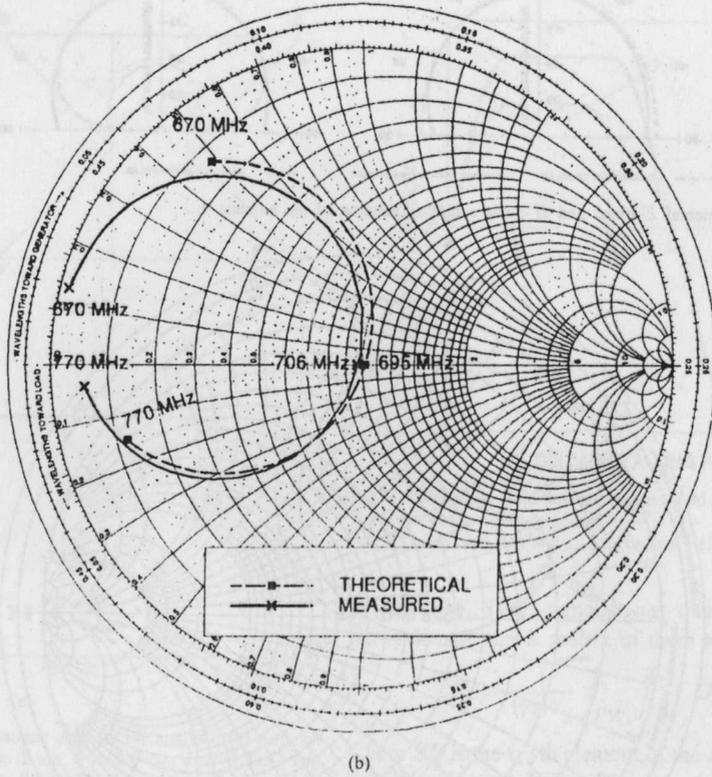
Fig. 7. (Continued.) Theoretical and experimental impedance loci of the antennas A, B, and C. (b) Antenna B.
