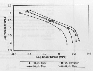
FIGURE 4 Shear viscosity versus shear stress at 80°C.
