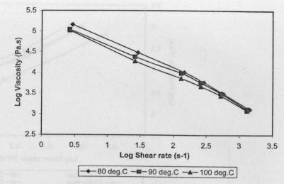
FIGURE 9 Shear viscosity versus shear rate for Mix D.
