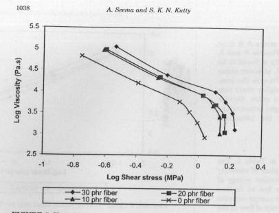
FIGURE 5 Shear viscosity versus shear stress at 90°C.
