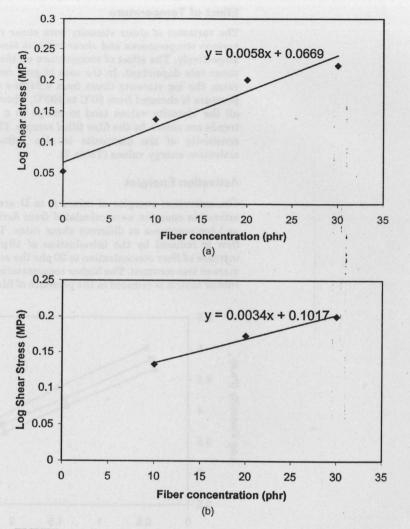
FIGURE 7 a) Variation of shear stress at the point of inflection with fiber loading at  $80^{\circ}$ C. b) Variation of shear stress at the point of inflection with fiber loading at  $90^{\circ}$ C.
