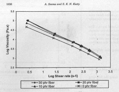
FIGURE 3 Shear viscosity versus shear rate at 100°C.
