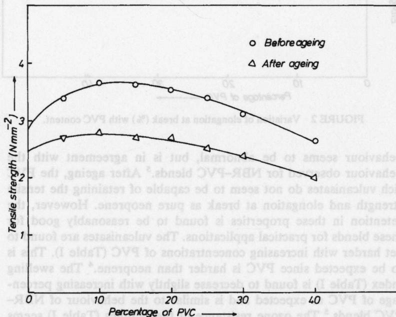
FIGURE 1 Variation of tensile strength with PVC content.
