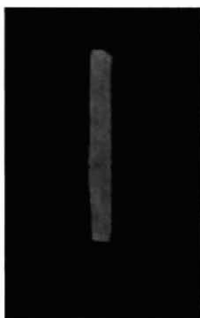
Figure 3.17: X-ray photograph of chitosan formate microspheres containing barium sulphate (filled in polyethylene tube)
