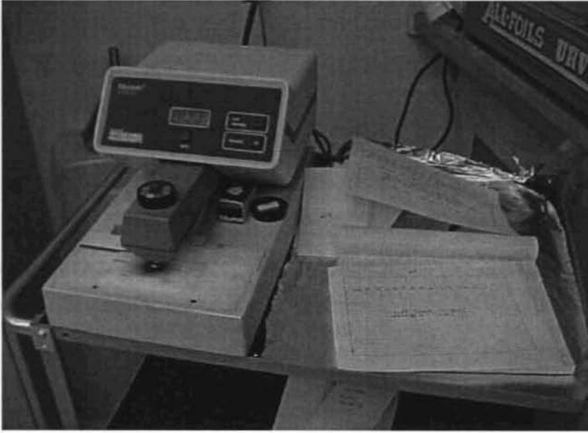
Figure 2.1: Densitometer used for optical density measurements
