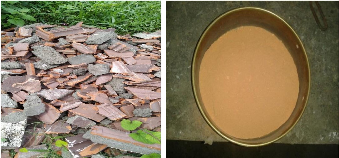
Fig 3.2: Broken roof tile and roof tile powder
