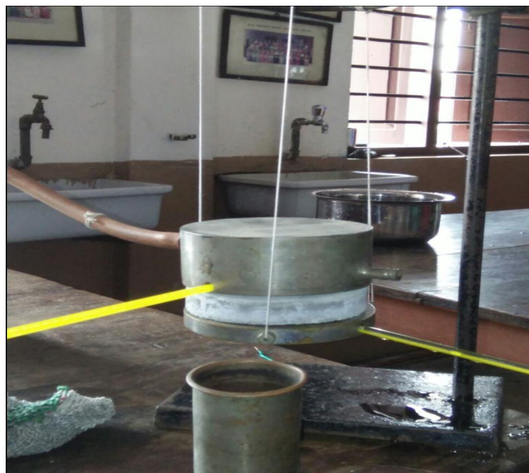
Fig.4.3: Experimental setup for thermal conductivity
