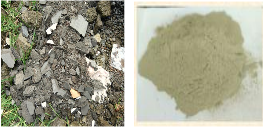
Fig 3.3: Demolished concrete and powdered concrete
