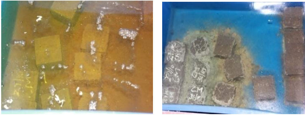
Fig. 4.6: Samples immersed in HCl and H 2 SO 4 at 150 days
