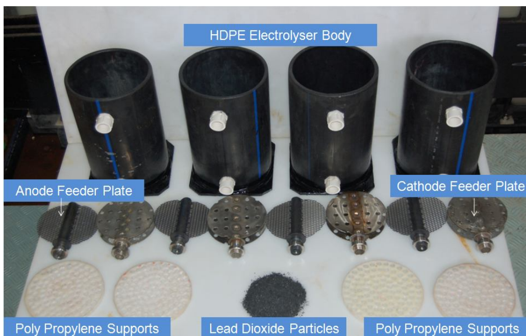
Fig.4.12 Major components fabricated for arrangement of single bed PBER's
