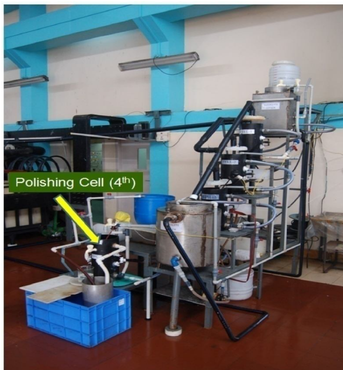
Fig.4.28 Modified orientation of 4 th cell (“Polishing cell”)
