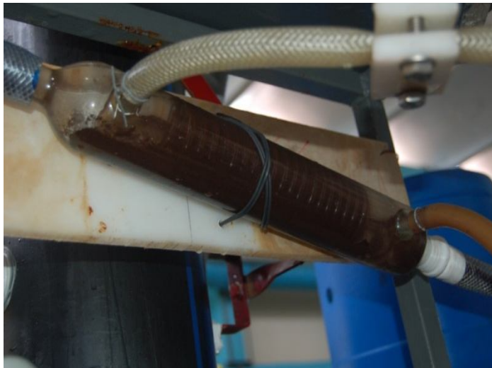
Fig.4.27 Line condensers inserted between cells
