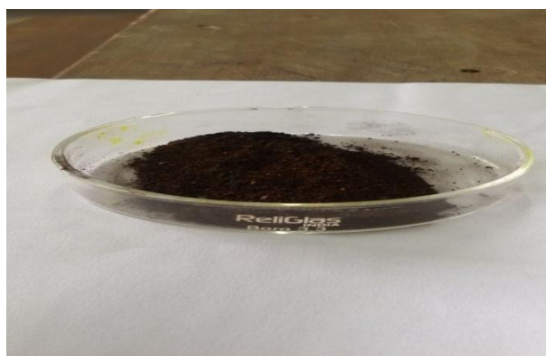
Fig. 3.2. Synthesized Fe-loaded chitosan nutmeg shell powder
