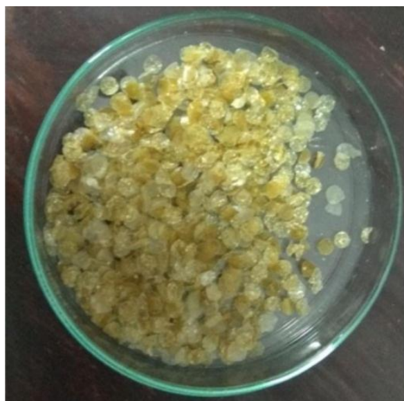
Fig. 3.3 Synthesized chitosan-bentonite nanocomposite films
