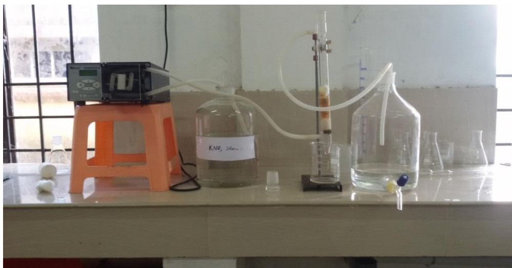
Fig. 3.7 Nitrate fixed bed column using CH-B-NCF
