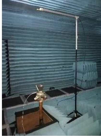
Figure 3.5. Axial ratio measurement setup
